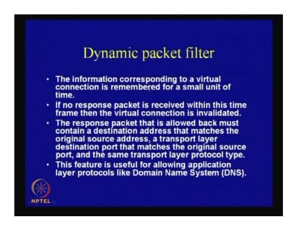
Therefore, they were not applicable for the UDP, but on the other hand, this is actually helping us to extend the security checks to the UDP networks and UDP protocols as well. So now, the information corresponding to a virtual connection is remembered for a small unit of time.
