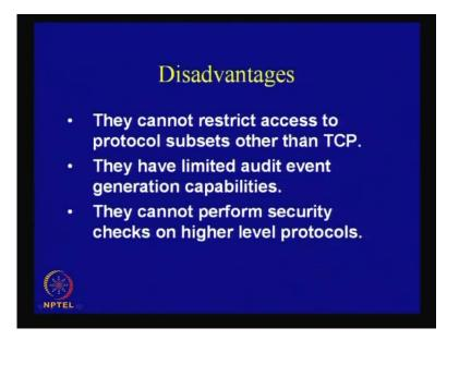
The disadvantages are it cannot restrict access to protocol subsets other than the TCP; it is only specified to TCP, they have got limited audit event generation capabilities; this is kind of limited, and they cannot perform security checks on higher level protocols; if you have got any higher level protocols then these are not meant for them.
