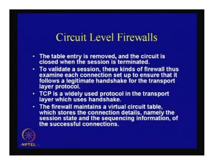
Now, this table entry is removed and the circuit is closed when the session is terminated to validate a session. These kinds of firewall thus examine each connection set up to ensure that it follows the legitimate handshake for the transport layer protocol. TCP is a widely used protocol and it actually uses handshake, and the firewall maintains the virtual circuit table which stores the connection details; namely the session state and the sequencing information of the successful connection.
