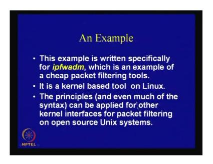
Now I give a brief example, this example is specifically written for ipfwadm, which is an example of a cheap packet filtering tool, and which is the kernel based tool on Linux. The principles and even much of the syntax can be applied for other kernel interfaces for packet filtering on any open source UNIX systems.
