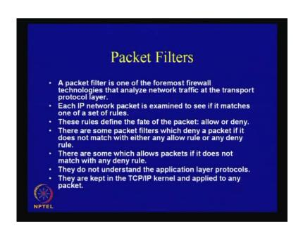
We will just have a quick look into what are these types of firewalls, and what is the basic principle of working of these firewalls. So, a packet filters are actually the foremost and most primitive technologies that analyze network traffics at the transport protocol layer. Each IP network package is examined to see if it matches a set of rules; these rules
