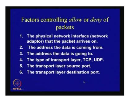
Now, typically the factors which controls the allow or deny of the packets are as follows: the physical network interface or the adapter that the packet arrives on, the address the data is coming from, the address the data is going to, the type of transport layer that is whether it is TCP or whether it is UDP, the transport layer source port, and the transport layer destination port.
