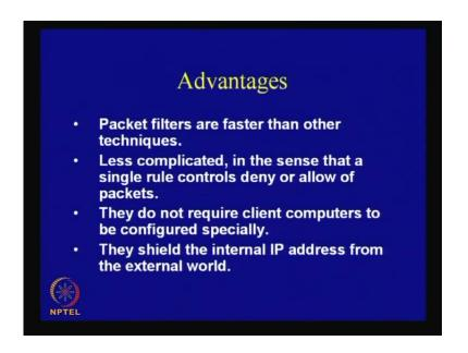
So, the advantages of the packet filters are, of course they are fast because they do minimize security check, and they are very less complicated. They do not require the client computers to be configured specially, and also they shield the internal IP addresses from the external world. Like you do not see exactly what is the internal IP address of the network when you are communicating with a network in the internal IP'S.
