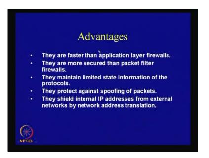
Now the advantages are, of course as you understand that they are faster than the application layer firewalls, they are more secured than the packet filter firewalls, they maintain limited state information, they maintain some amount of sequencing information, they protect against spoofing of the packets, they also shield internal IP addresses from the external networks by performing the network address translation. These are some of the advantages.
