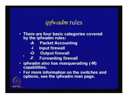
So here is an example, I would not go much but if you do a man of this ipfwadm, then you will see that these are some of the basic switches which you have like the packet accounting, input firewall, output firewall, and the forwarding firewall. There are lots of other switches also, like you can also mention masquerading capabilities. So, for other information on the switches you can actually see the corresponding man page.
