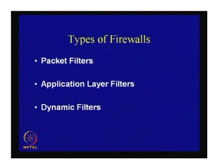
So, these guards are technically known as the firewalls. Typically, there are three kinds of firewalls which are used, so the three types of firewalls are known as the packet filters, application layer filters, and dynamic filters.
