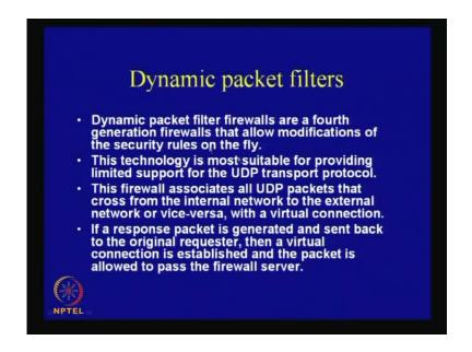
Therefore, if there is no response during this time then within the time frame the virtual connection is invalidated. In these kinds of dynamic packet or this kind of filters, in dynamic packet filters if the response packet is generated and sent back to the original requester then a virtual connection is established and the packets are allowed to pass the firewall server.
