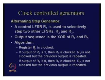
We will rather a little bit concentrate upon something, which is quite interesting, called as Clock controlled generators. There are two types of clock controlled generators, one: which is called an Alternating Step Generator. What is the construction principle? There are essentially three LFSRs here, say control LFSR R 1 is used to selectively step two other LFSRs, R 2 and R 3.
