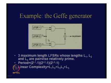
Let us, consider one simple example this is something which is called the geffe generator. There are three LFSRs here and this is producing one output, this is producing one output, this is producing one output and this is the key stream therefore, you can see that this is particular if, I box this one then this is my f and what is the form of f? You take x 1 you take x 2 add them so it is x 1 x two xored with x 3 x 2 bar.
