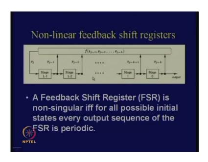
First of all, let us start with non-linear feedback shift registers. As the diagram says that, it is exactly the same as that of feedback shift register which we have already seen but, only the difference is, in this case your feedback is non-linear.
