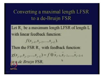
In that case, I know how to produce a three bit maximal length LFSR? How can I modify to obtain a such a de bruijn generators, this is how you can do it and its quite simple to follow. In order to convert, say that let R 1 be a maximal length LFSR of length L with linear feedback function fsj minus 1 sj minus 2 and so on till sj minus L therefore, this is an maximal length LFSR.
