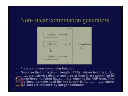
Let us consider this; suppose there are n LFSRs and all these LFSRs are producing a key stream. What we do next is that we take a function f and we combine all of them and produce a key stream note, that here f is a non-linear combining function, suppose there is a result which states like this, that n maximal length LFSRs all of them are maximal length LFSRs and then lengths of all of them are say L 1, L 2, and so on till L n where, L 1 to L n are all mutually co-prime.
