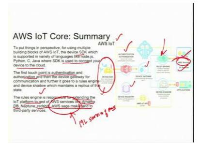
So, let us summarize about AWS IoT core architecture. So, put the things in the perspective for using the multiple building blocks of AWS IoT core. That is the device SDK, which is supported in a variety of languages, and it is used to write a application for the devices. And these devices allows the SDKs to connect to the cloud.
