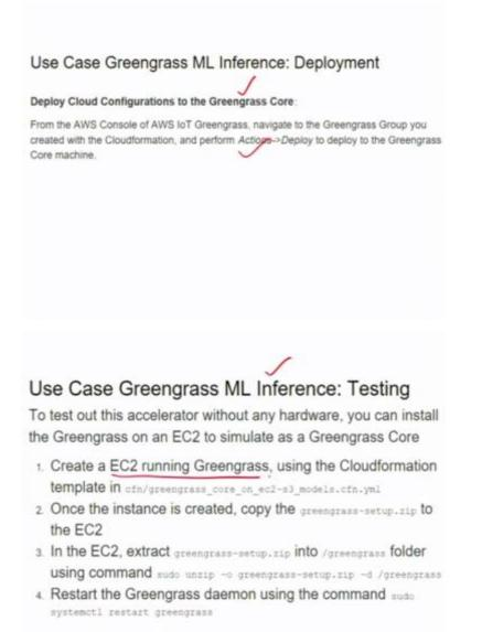
So, then once the model is trained in the sage maker or in the, in the cloud AWS cloud, then it will be deployed using the Greengrass group into the, the Greengrass core. So, this is the use case of a Greengrass machine learning inference: testing. So, you have to create the easy two running instance running the Greengrass, and then it will deploy all that command.
