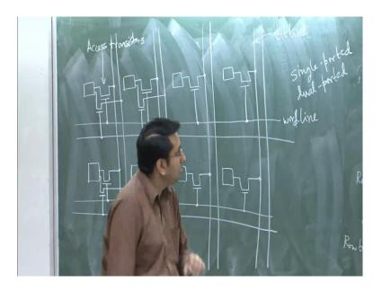
Showing 1 more example, so I will show you 2 rows of the D RAM first show you how it works. So, these are more bit rows that I am showing that often 2 rows of D RAM this is the D RAM cell which stores the bit all right. And this is the switch all right which closes whenever I give a high voltage here on this particular wire all right. Whenever I give a high voltage here this closes and what about the value of this here will appear on this particular wire all right.
