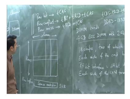
This 1 is called sense amplifier as a technical name if you want to read up on that I can give you some references. So, a narrowing of sense amplifiers actually hold the data gets the row buffer and then it involves a lot of electrical engineering how to design good senses in sense amplifier refresh data is I already talked about. So, periodically the memory controller which scheduling refreshes cycle is on the other hand.
