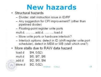
So, whenever I have a division instruction I will check if, currently there is anything in the divider; that is it can be easily maintained here. So, that I can stall the instruction. So, clearly that is going to introduce bubbles in my pipeline. So, a slightly smarter thing that I could have done here, is that I can only stall the instructions.
