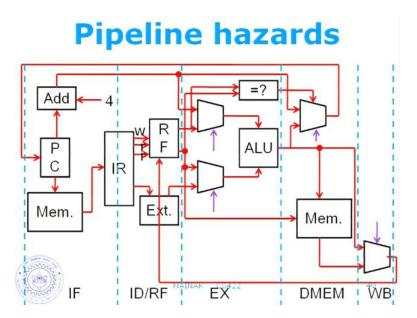
And there is a Mem to ex also. So, there will be two multiplexers, each accepting two inputs from bypass, and one from a register file .If I ignore the write back to ex bypass for now. And the Mem stage will have just one bypass part for now. We will come back to write back to Mem bypass very soon, and there will be one multiplexer. So, that is in
