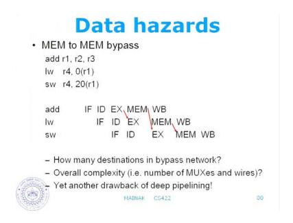
And we are selecting to this and this in a register cycle, based on the comparison of the register identifiers. In this case I will be comparing r 4 by the destination of this 1, and though they match, so I will say I have to take the bypass now. So, as you make the pipeline deeper, you need more and more bypass pass.
