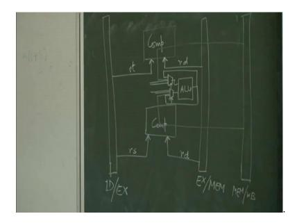
So, it tells me a answer; the comparator r. I need to override the inputs to the A L U, this one is wrong, this one could be wrong, both could be wrong, one could be wrong, both could be correct.
