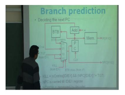
Here it is ((Refer Time: 24:24)) So, this is the program counter. And, this is actually the pipeline register at the front of the fetch stage. So, here I show this in a dotted line; it is
