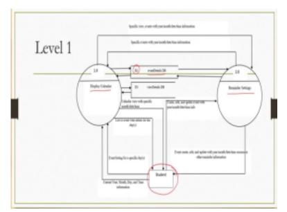
So, earlier we saw Display calendar process. Now, there can be another reminder settings process at the same level 1. Now, this process interacts with D2 event details database. But not with D1, view details database. As well as, it interacts with the external entity and the other process as shown in this figure, are these the only 2 let us see
