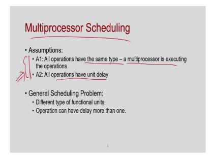
So, in the multiprocessor scheduling, we have certain assumptions; so, on these four parameters. We assume that this particular all operation of the same type; that means, there is a multiprocessor which can execute this operation. So, that means, although this nodes can be plus, minus, multiplication, division; but you can assume there is a kind of processor which can perform any operation.
