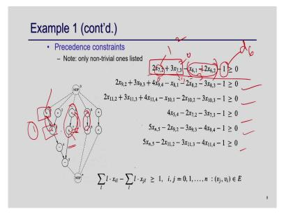
For the precedence constraint, it is basically for every edge. So, if you just take an edge here, so this is I have to check the possible start time of this and the possible start time of this, but the difference will be 1 because the this operation has a delay 1 now. So, what are the possible start times of this node say 7? So, let me take this example. So, 7 can start here or here, without touching the delay and if 7 work here, the 6 can come here.
