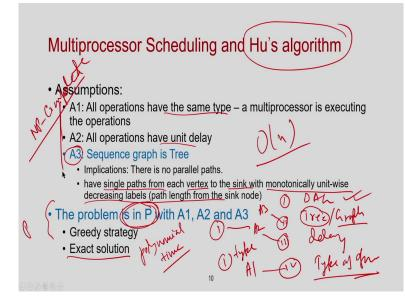
So, as I mentioned in the start of the class that the objective of this class to identify a sub class of my sequence graph which is polynomial time solvable and if we assume this the graph has all operations of same types that there is no different types that I have already assumed and the all operations have unit delay, still this problem is NP complete. So, even if this particular two assumptions are there, still these problems are NP complete.
