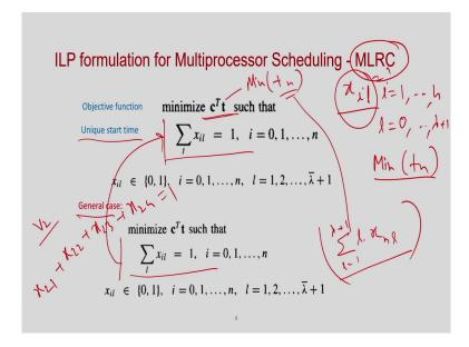
So, you if you remember that this ILP formulation, we have taken a variable called x il, so which is basically because what is our objective i? Our objective is to identify the time step, where this operation is going to start its execution and that is unknown. So, I have just taken a variable this i l; where, i varies from 1 to n representing the nodes and l representing the time step, which is basically 0 to lambda plus 1.
