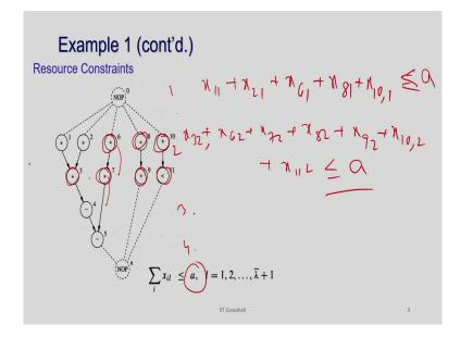
And for resource constraint is basically I have to see what are the node that can be schedule in time step 1 because ah. So, what is the node can schedule in time step 1? So, 1, 2, 6, 8 and 10. So, that means, x 11 plus x 21 plus x 61 plus x 81 plus x 10 1 should be less than equal to t; it should be less than equal to a. Because this is the resource bound.
