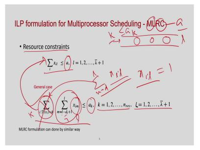
So, now, I will move on to the next constraint. In the next constraint was the resource constraint, you remember and the resource constraint says that in each time step, the number of operation that are running in that time step of set 1 type of resource k must be less than a k; that means, the number of resource available of type k.
