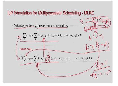
So, next one was the precedence constraint or data dependency. So, if you remember that if there is an edge from v j to v i and this node has a delay of d j, then what is the idea that if this is schedule in t j and it will take say till t j plus d j minus 1. So, it will execute in this time step. So, the t i the time step of this t i must be greater than equal to t j plus d j, that we have understood and we can represent this t j, this t i by this and t j by this.
