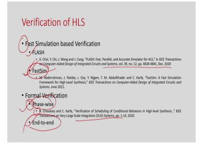
Another very important, very active area of research is verification of high level synthesis. So, we have seen that whenever we generate RTL from a C code; because of the completely different semantics, different ways of execution of those behaviors. So, checking functionality whether the generator RTL is functionally equivalent to the input C code or not is extremely important. So, there may be some bugs introduced for many reasons.
