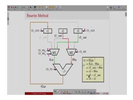
So, suppose this is the data path and these are the control signals are there in the data path that is the value will come from the controller and say in one clock, you actually give these values to the controller some 1 0 values. As a result, only few of the operations will be active.
