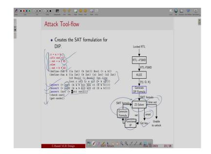
Then, I am going to give the things to the SMT solver. So, we have used tool call Z3 to generate this and then, what will happen? Those SMT will basically identify a DIP and then, I will just evaluate that with the DIP that actually oracle and then, I will get a constraint which is the next formula and we will update that formula, we just add this formula and again I am just going to call this Z3 solver. This is the things whole things going to happen iteratively.
