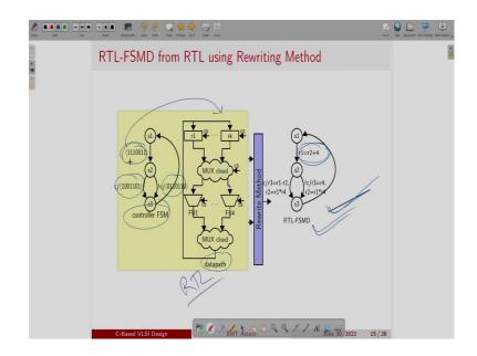
So, I can apply that RTL to C reverse engineering technique and I can actually extract a high-level behavior. Just to recap what we have done actually is you have that RTL; this is the RTL that is generated by high level synthesis tool which has a separable controller and data path that I have already discussed.
