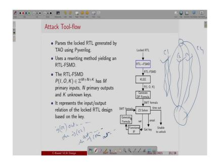
Then, I have used a tool called KLEE, which is basically symbolic simulator tool which will give you the all the paths of your program. So, in a program what is going to happen? There are many paths. So, and each path has a condition and you have set of operation is happening. So, KLEE will identify all the paths in your program and we assume the loop is basically static. So, KLEE will unroll the loop.
