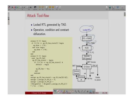
So, only thing is remaining to be discuss is that how do we model a program. So, this is the overall tool flow, we model the program symbolically. So, we have the RTL. Using my RTL to C converter, I get an RTL-FSMD.
