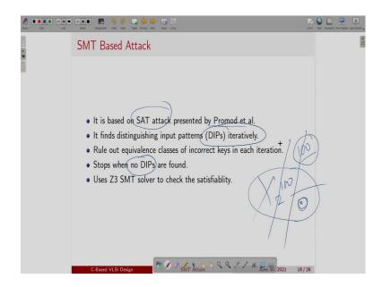
So, I am going to break these three kinds of techniques using a technique called SMT based attack. So, from the RTL, I abstract out of an FSMD and then, I am going to launch the attack that is what the overall process.
