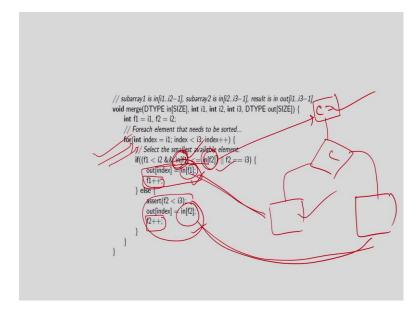
So, now once you apply this you will notice that you will not get I I equal to 1, if even if you apply this loop unroll and pipeline, specifically the pipeline to this loops innermost loops specifically the innermost loop and it says that I am not able to generate the II is equal to 1 because of this reason. So, it will give you some reasons right.
