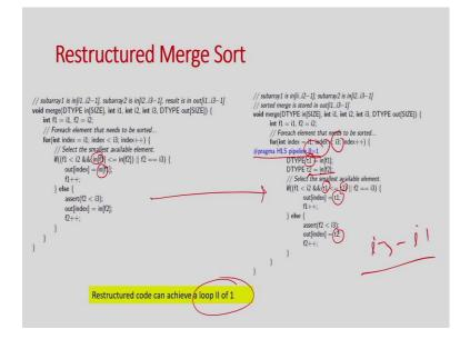
So, the suggestion is I already mentioned that I am going to I am not going to read this way. I just read this in f1 and I will store in a temporary variable. I will read in f2 and store in a temporary variable t 2. And everywhere instead of using a this in 1 and in 2, I am going to use t1 t2. I am going to use t1 or t2. So, that is all my problem because I do not have four reads.
