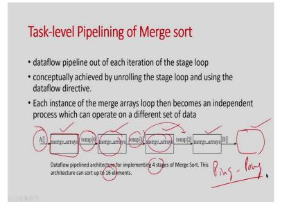
And so, let us try to understand that what I can do is basically you have to create a data flow things right. So, as I mentioned I give the array A and then here this merge by one is happening.
