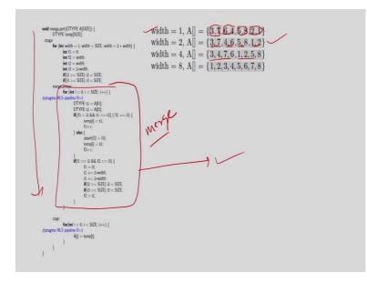
So, basically what is happening here is so, whenever I give this the first block will try to merge these two array into 1, these two array into 1 these two array. So, all these things will going to happen, but this block will do this operations and it will give you this array right where this each two elements are sorted ok.
