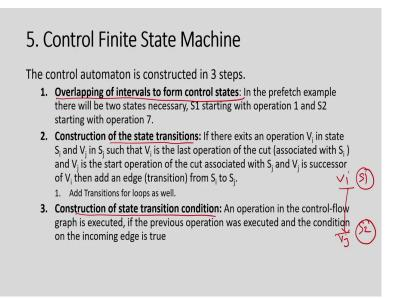
So, as I mentioned that, I have identified the states; the now the find is that, you how you identify the overlapping of interval to form the control state. So, that is already done, you identify the overlapping and this is my control state 1. And then you, so and similarly this is my control state 2, which is the overlapping of these three cuts.
