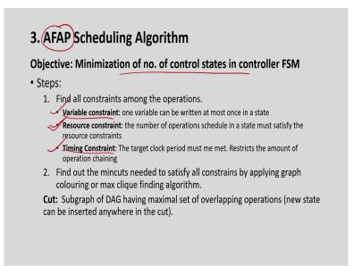
So, the idea of this scheduling is the AFAP algorithm. So, the idea of this algorithm is to minimization of the number of control states. So, there are two steps primarily in this algorithm. So, basically you have the operation in the particular path; what I am going to do? I am going to identify the constraint, what is the kind of constraint the schedules should satisfy in this path.
