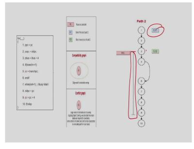
So, if you take the path 2, you also identify there are two cuts needed. So, this is one cut and this is another cut; in this case I have only one constraint.
