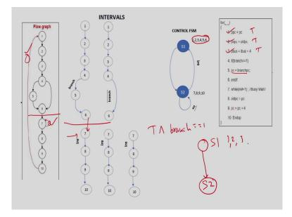
So, suppose I am in this state S1 and I want to go to there is a state S2, I have a transition here. So, I am going to have this transition once these operations are all done. So, if there is a 1, 2, 3, these three operations are done. So, that means the condition should be AND of condition of all these operations. So; that means, the AND of whatever the condition for this operations that should be added.
