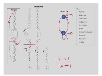
So, you can understand here that I cut the path here. So, basically at this point; so that means operations 1 to 6 is going to happen in state 1 and operations 7 to 10 is going to happen in state 2. So, that means in state 1, I am going to do this operation as well as the if else part; in state 2 I am going to perform this while loop as well as the operations following the while loop. So, this part we understood and this is what is already done.
