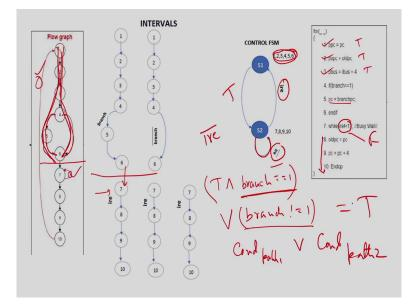
So, now for this branch, the condition is basically branch bar. So, branch basically not equal to 1, then only you will shape it. Since this if and else both the branch is happening here, so the condition should be OR of this. So, that means if you look into this program; the idea is that you identify the number of paths, there are two paths here.
