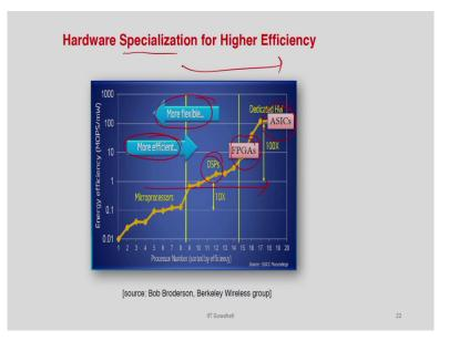
And, this specialized hardware has advantages and disadvantages. So, whenever you have a general purpose processor, it is more flexible, right. So, you can actually have a processor which can do image processing, it can do some AI things, it can do anything, right. It can actually do some video coding decoding and whatever it is. It can do anything right as long as you can map these things into the instruction set. So, it is more flexible, but it is less efficient, right.
