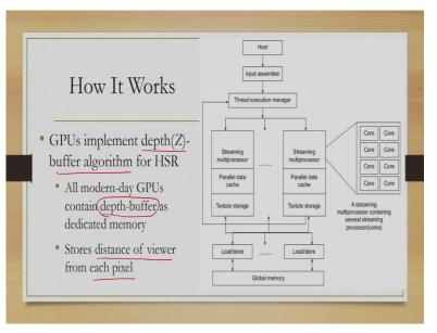
Also, we discussed earlier during our discussion on hidden surface removal, the idea of Z buffer algorithm or depth buffer algorithm. Now, that is implemented in GPUs and for that also typically GPUs are equipped with specialized memory element or depth buffers. And it stores distance of viewers from each pixel. So, that is typically part of the GPU.
