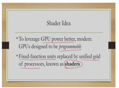
But then people realize that, that is actually reducing flexibility and because of that power of GPU was not fully utilized. To leverage the GPU power better, modern GPUs are designed to be programmable that means we can program them. Fixed function units are replaced by unified grid of processors known as shaders. So, earlier there were fixed function units, now there are unified grid of processors which are called shaders.
