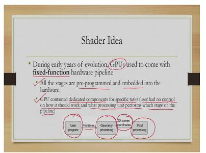
Now, during the early years of GPUs they used to come with fixed function hardware pipeline, that means all the pipeline stages or all the stages that implement the pipeline are pre-programmed and embedded into the hardware. GPU content dedicated components for specific tasks and the user had no control on how this task should be performed and what processing unit performs which stage of the pipeline.
