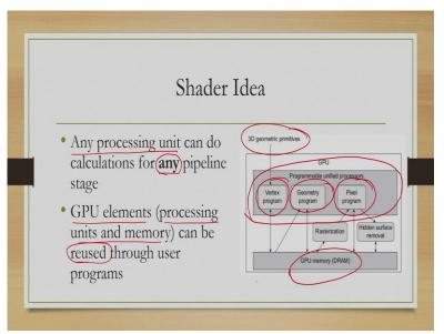
And any processing unit can be used for performing any pipeline stage calculation. And the GPU elements, that is the processing units and memory can be reused through user programs.
