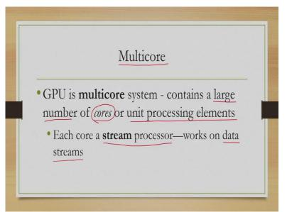
Let us go into the workings of GPU. Now, we have to note that GPU is a multicore system that means it contains a large number of cores or unit processing elements. Now, each of these cores or these unit processing elements is called a stream processor. Because it works on data streams, streams of input data.
