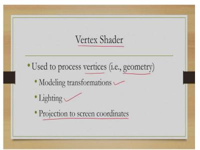
In case of vertex shader, what happens is that, these programs are used to process vertices or the geometry. Essentially these programmes are used to perform modeling transformations, lighting and projection to screen coordinates which involve all the intermediate transformations of view transformation. And conceptually the window to view put transformation as well.
