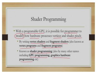
Now, with the programable GPU that we have just introduced it is possible for programmer to modify how the GPU hardware processes vertices and shades pixels, shades means assigns colour to the pixels.
