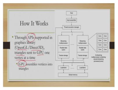
Now, given that triangular mesh information what happens is that, those dedicated APIs which are provided in the graphics library such as OpenGL or Direct3D, these triangles are send to GPU, one vertex at a time serially and GPU assembles them into triangles.
