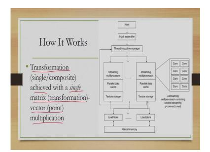
And so we are dealing here with the very first stage that is object definition, so these objects are defined in their local or modeling coordinate systems. Then the GPU performs all the stages, so first it performs modeling transformation on vertices that is the first stage of processing.
