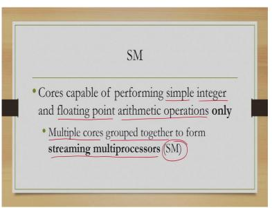
Now, these cores are nothing but simple hardware capable of performing simple integer and floating-point arithmetic operations only. So, each core can perform arithmetic operations only, either integer arithmetic or floating point arithmetic. And multiple cores are grouped together to form another unit called streaming multiprocessors or SM. So, each core is called
