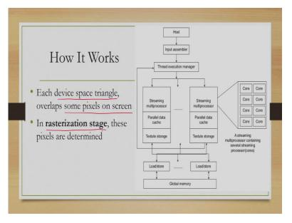
So, after that stage we get the device space triangles and we now go for rasterization or scan conversion. So here it may be noted that each device space triangle overlaps some pixels on the screen that means those pixels are part of the triangles. In the rasterization stage these pixels are determined.
