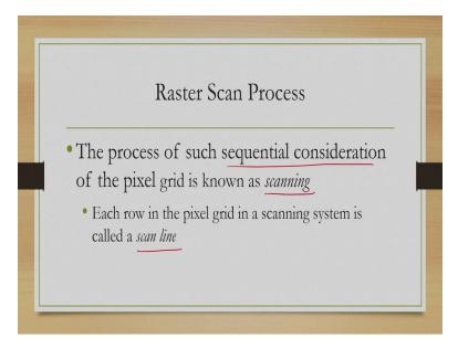
Now this process of consideration of pixels in sequence or such sequential consideration of pixels is known as scanning this is a more generic term used that in raster scan devices, pixel scanning takes place each row of the grid is known as a scan line. So this sequential consideration is called scanning and each row in the pixel grid is known as scanline.
