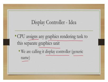
And the CPU as science any graphics rendering task to this separate graphics unit and we call this graphic unit as the display controller which is a of course generic name and in different systems it is called in different ways. So essentially display controller deals with performing the multi-stage operations required to create or synthesize a 2D image.
