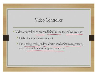
So what it does? It essentially converts digital image that is represented in the form of 0's and 1's to analogue voltages, why? Because the voltages drive electromechanical arrangements which ultimately render image on the screen. So screen essentially is a electro mechanical mechanism and to run this mechanism we require voltage and this voltage is generated by the video controller based on the 0's and 1's stored to represent the image.
