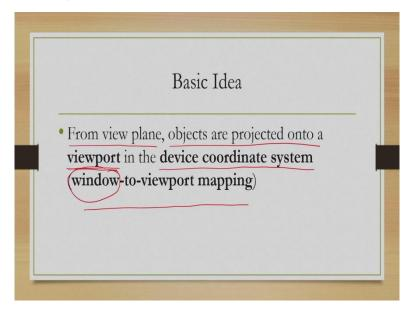
Now, from the view plane after projection, we perform another transformation. The projection is done on a viewport on the view plane. Now, from there, we transform the objects into the description on a device coordinate system. So, when we perform projection transformation, we essentially transform on the view plane. Now, that area where the image is projected is called the window.
