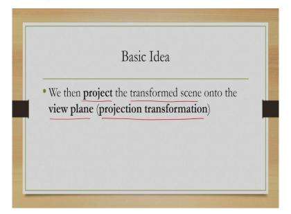
Then we project the transformed scene onto the view plane. So, this is the projection transformation, so first comes 3D view transformation, then comes projection transformation.
