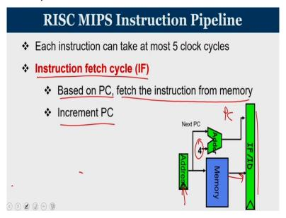
So, the first one is known as instruction Fetch, this is the circuitry associated with the instruction fetch. What it does is based on the program counter value fetch the instruction from memory. So, this is the address that has been supplied by the program counter, it goes to the instruction memory or memory in which the instruction is been stored and the contents of that is been taken and that has been stored in the pipeline that IS / ID.
