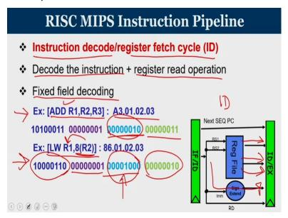
Now, moving on to the second stage, the second stage is also known as instruction decode as well as register fetch cycle which is abbreviated as ID. So, whatever you have done in the instruction fetch stage, an instruction is available in the IF/ID register. And from there, you do some operation at the end of this unit the ID/EX register will contain the resultant of the decoding and register fetch operation.
