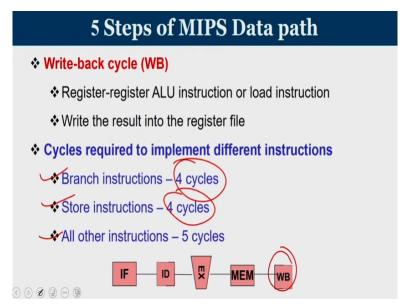
And the write back stage writes the result of an operation that has to be reflected inside a register. So, in short branches will typically get over in 4 cycles, stores also will get over in 4 cycles or other instruction will go to the fifth cycle where in a write back is happening.
