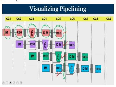
This is yet another visualization of the pipeline. Previously we were telling what are the operations to be done here this diagram shows which are the functional unit that are busy. First
