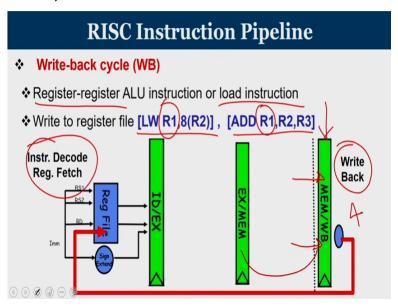
The next is the fourth stage, it is also known as memory access cycle called MEM stage this stage is used only by load and store instruction if it is a ALU instruction, then no operation is carried out in the MEM stage, whatever was the result that was available in EX/MEM register, that is simply by passing into the MEM right back register, if it is a ALU operation, if it is a load
