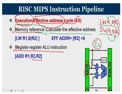
In any case, the values will reach the ID/EX register. Now, the third stage is known as execution stage, it is also known as effective address stage. The abbreviation given to the stage is EX. The operation that is carried out in the EX will vary depending upon what is the operation? Consider the case that the operation is a memory reference that it can be a load word operation or a store word operation.
