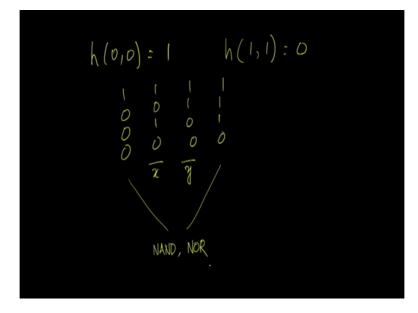
If this is a universal logic gate then when both the inputs are 0, the output of h will have to be 1 otherwise we will not be able to use h to synthesize a function like NAND that is because when you have a circuit made up only of h gates and when both the inputs to the circuit are 0 then the circuit will have only 0s in the inside, if h of 0, 0 were 0. Therefore, to be able to synthesize every function which produces 1 when both the inputs are 0 h of 0, 0 will have to be 1.
