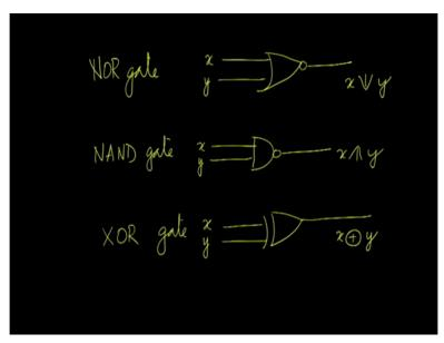
A NOR gate, which is a negation of OR is drawn in this manner, x and y are the inputs the output is x NOR y and NAND gate, is an AND gate followed by a negation, an XOR gate, which produces an output of 1 if and only if the inputs are not the same, it is denote it like this. Therefore, using these logical gates you can convert a Boolean expression into a circuit.
