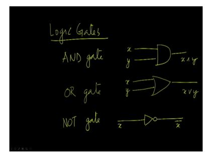
Some of these logical connectives can be expressed as logic gates and, AND gate is drawn like this in a circuit diagram. So, an AND gate has 2 inputs x and y and the output is x and y, the output is 1 if and only if both the inputs are 1. An OR gate is represented in a diagram in this manner where the inputs are x and y and NOT gate has only 1 input, let us call it x and its output is the negation of x.
