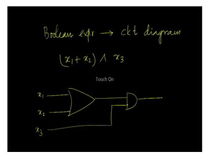
For example, if you have a Boolean expression of this form, we have the signals  $x \ 1$  and  $x \ 2$  they can be odd using an OR gate, the output of which can be ANDed with  $x \ 3$ . So, this is the circuit diagram corresponding to this Boolean expression. So, what we know is that any Boolean expression can be converted into a circuit diagram using AND, OR, NOT gates, using either the sum of products form or the product of sums form.
