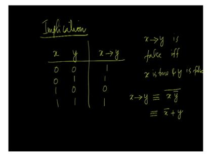
Now, let us consider implication. The implication is a 2 variable Boolean function with this truth table, when both the inputs are 0 the output is 1, when x is 0 and y is 1 the output is 1, when x is 1 and y is 0 the output is 0 and when both the inputs are 1 the output is 1. So, what it means is that, x implies y is false if and only if x is true and y is false or we can say, x implies y is logically equivalent to the complement of x y bar which by De Morgan's law is x bar plus y.
