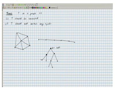
So trees are graphs, which has two crucial properties. So let us call it by T. So t also there is a graph first requirement is T should be connected. The second requirement is that T should not contain any cycle. So let us see some examples if you look at this graph on 6 vertices this is called as star graph. So this graph does not have any cycles and it is a connected graph. It is a line graph this is also an example of a tree.
