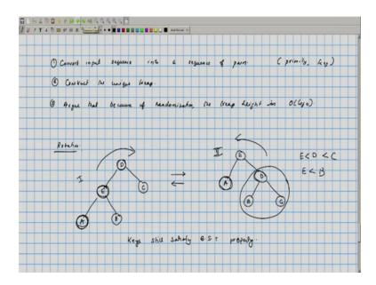
So, in a nutshell what we will do is convert input sequence which was a sequence of integers into a sequence of pairs ok. So, if the input if you think of them as keys, we will convert it into priority key pair and then we will construct the unique treap if you are introducing a new element that will also result in a unique treap which can be incrementally computed from the existing treap and then we will argue, that because of randomization the treap height is bounded by o log n ok.
