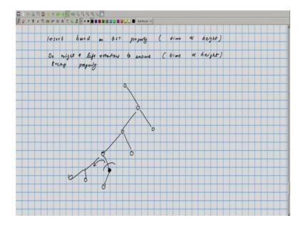
Insert based on BST property, when you do this the time taken will be proportional to the height and once you have inserted a particular pair the tree property need not be maintained. So, we will do appropriate right and left rotations to ensure treap property.
