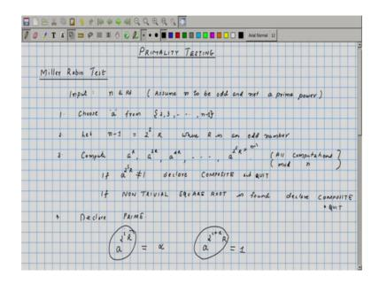
So, the steps in Miller Rabin are as follows, if the so we will assume that the input as a an odd number and not a prime power. We choose a random a and compute a raised to R, a raised 2R, a raised to 4R and so on, up to a raised to 2 to the S R 2 to the S R is equal to n minus 1.
