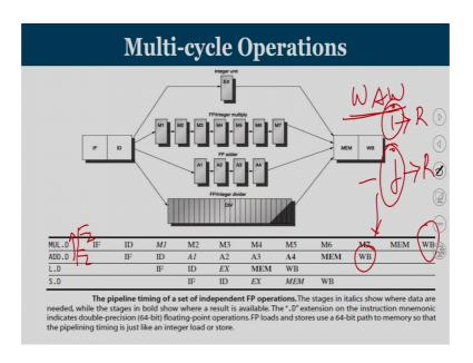
So, consider the case that let us say you are going to write on a number add is going to, let say add is going to write on the register F 2 and multiplication is also going to write on a register F 2, add is issued after the multiplication add comes after multiplication because of long multiplication stage multiplication get over only here whereas, adding gets only will be done before that.
