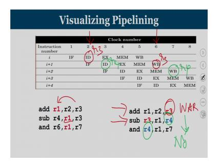
So, when we work on WAR hazard, these are typical cases of WAR hazards right after read, you are going to read from r 3 that happens here in the second clock cycle and you are going to write the value into r 3 and that happens here.
