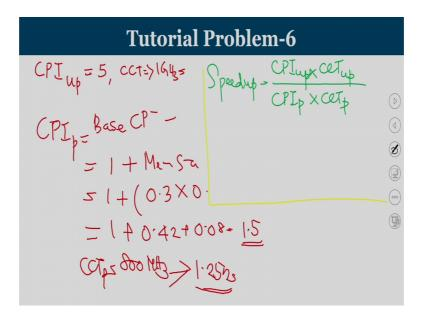
So, speed up can be defined as CPI of the unpipelined into clock cycle time of unpipelined divided by CPI of the pipelined processor into clock cycle time of the pipelined. So, if the clock cycle time of the pipeline is going to be larger because for implementing a pipeline you have to add the interface registers.
