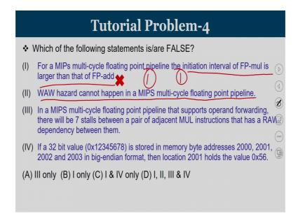
So, the statement for a MIPS multi cycle floating point pipeline initiation interval of floating point MUL is larger than that of floating point add is wrong because both has initiation interval of one. So, statement number 1 is false. Look at statement number 2, WAW hazard cannot happen in MIPS multicycle floating point pipeline, what you mean by WAW hazard write after write hazard if the second instruction is going to write on a value where the first instruction is also going to write.
