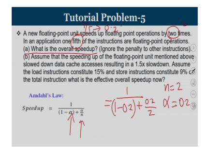
Now we are moving into the fifth problem, this problem has two sub divisions, a new floating point units speeds up floating point operations by two times in an application one fifth of the instructions are floating point operation what is the overall speed up. So, we have to understand that your floating point unit is going to improve your performance by 2 times.
