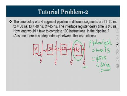
Now, I request you to consider the second problem. This is an pipeline associated problem, time delay of a four segment pipeline in different segments are t 1 equal to 35 nanoseconds, t 2 is equal to 30 nanoseconds, t 3 is equal to 40 nanosecond then the t 4 is equal to 45 nanosecond. The interface register delay time is t equal to 5 nanosecond. How long would you take to complete 100 instructions in the pipeline? Assume there is no dependency between the instructions.
