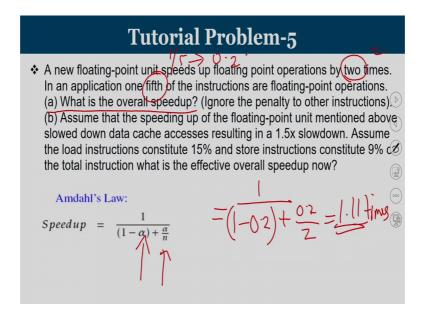
So, when you use a floating point unit that is going to improve the performance by two times for floating point instructions, let us say the floating point instruction is only 1 by 5th of the total instruction then what is a overall speed up, the overall speed up is 1.11 times.
