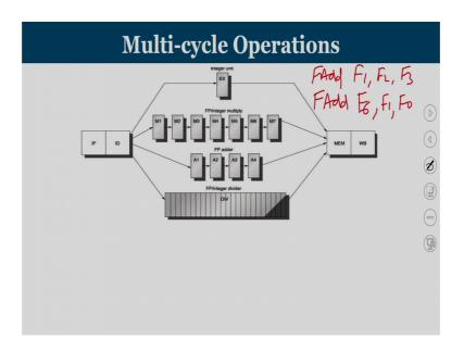
So, this is the floating point the pipeline. Now we are going to talk about a case where two adjacent adding operation let us say we are going to add two floating point numbers F 1, F 2 and F 3 are going to be add. So, the result is going to be obtained in F 1.
