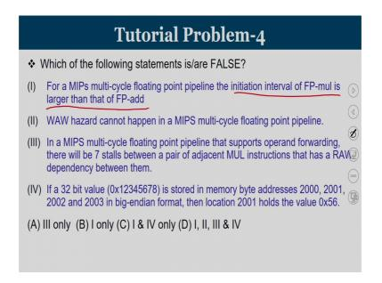
Now, we have one more true or false case, which of the following statements are False? For a MIPS multi cycle floating point pipeline the initiation interval of floating point multiplication is larger than floating point addition. So, how will you tackle this statement? There is a floating point multiplication which we have seen that it has 7 pipeline stages; M 1, M 2, M 3, M 4, M 5 like that these is the floating point pipeline, M 1 to M 7 and floating point adding as A 1, A 2, A 3, A 4.
