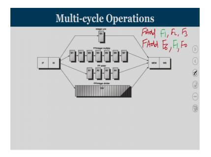
So, the first instruction is going to write into F 1, second instruction is going to read from F 1, now if you look at in a MIPS multicycle floating point pipeline that is supports operand forwarding there will be 7 stalls between a pair of adjacent multiplication instruction that has a RAW dependency between them.
