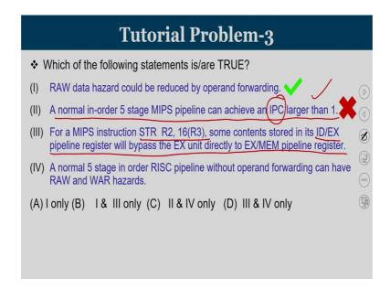
So, the statement is mentioning that a normal in order 5 stage MIPS pipeline can achieve an IPC larger than 1, Instruction Per Cycle larger than 1. Can we complete more than 1 instructions per clock cycle? That is not possible in the case of an in order 5 stage pipeline, such cases are possible only if it is an out of order superscalar pipeline. So, the second statement is faults.
