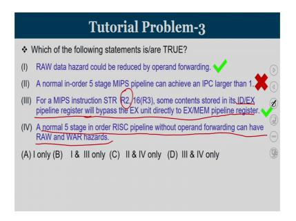
Now, if you look at, will bypass the EX unit directly to the EX MEM. So, from the ID EX pipeline register, the value of R 2 is going to bypass the EX unit, the value of R 2 will not go to the EX unit that is what we are going to see. So, this is true.
