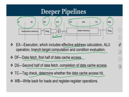
Coming into the subsequent stage the EX stage will take care of your normal execution, if it is an ALU operation, or if it is a load or a store operation it computes the effective address. If it is a branch instruction, then it computes the branch target computation and condition evaluation.
