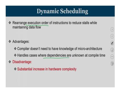
Dynamic scheduling is rearranging the execution order. And no longer rearranging the instruction, the instructions are in sequence, but rearranging the execution order of instructions to reduce stalls while maintaining the data flow.
