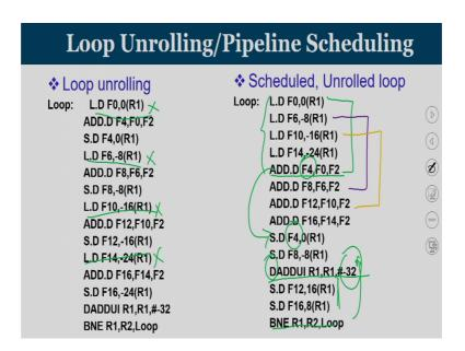
So, this is the unrolled loop. These are the places where we are going to have stalls. Now if you unrolled a code all the loads are been put together, all these loads are going to be put together, and the load and adds the corresponding adds this is the corresponding add when you work on this load and this add is 1. Now if I put this load and the second add is another 1, the third one is going to be dependent on the.
