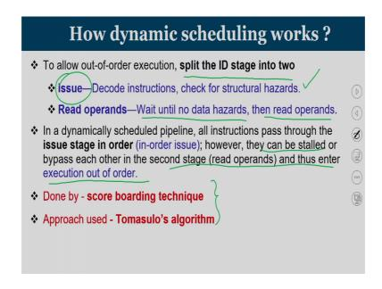
So, how dynamic scheduling works. To allow out of order execution we have to split the ID. The second stage into 2, one is called a issue stage, where you perform decode the instruction and check for structural hazards. So, if you have a structural hazard; that means, your functional unit is already busy, I cannot complete issue. So, completion of issue means decoding is over and there is no structural hazard on the functional unit where you are going to run the task.
