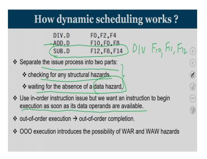
So, consider this case how dynamic scheduling is going to work the problem is a subtraction instruction which is independent which is not having any data dependency, maybe subtractor is free. So, there is no structural hazard, there is no data dependency then why should the subtractor be waiting.
