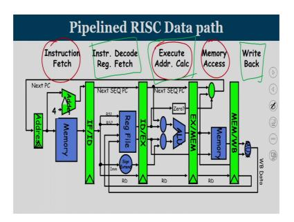
This is the conventional 5 stage architecture of the RISC instruction pipeline that we have seen; where, you have an instruction fetch stage followed by an instruction decode stage, and then we have the execute stage, memory access stage and the write back stage. The basic assumption that drives this 5 stage pipeline operation is, that we need only 1
