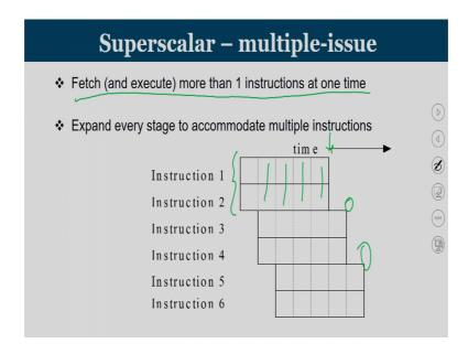
Now, coming to what are superscalar processors. With the normal processors with the instruction pipeline so far we have learned; we are fetching only one instruction. So, at most one instruction is going to complete and the CPI what we are targeting Cycles Per Instruction is 1; that means, with a normal scalar pipeline. We are trying to achieve one instruction getting over in every clock cycle.
