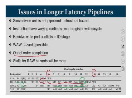
The first issue is a structural hazard. Since your floating point division unit is not pipelined; that means, for next 24 cycles, no other operation can use your functional unit, your division functional unit.
