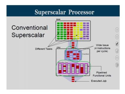
So, a superscalar processor means multiple instructions are fetched; multiple instructions are decoded, at the same time multiple instructions are also in execution.
