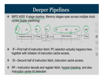
Now we will take one classical example of a deeper pipeline. Here we are going to work with MIPS 4000 pipeline it is having 8 different stages. So, these are the 8 stages you have 2 stages to fetch the instructions. Then you are going to have the decode stage which is also known as reading from the register. The EX stage then you have 3 stages for accessing the memory, and one stage for the write back.
