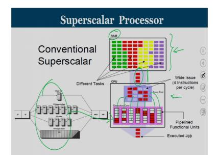
Now this is like conventional superscalar processor. This is a logical view of a superscalar processor. This different colour indicates different programs which is stored inside your main memory. So, you have different programs, you are going to fetch multiple instructions together into the processor. This is your memory and this is our processor.
