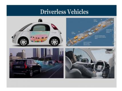
Now, in driverless vehicles, we know the concept of driverless vehicles, we have lot of sensors that is been fitted in the vehicles that are going to capture lot of information like, how far or close is the next object the next vehicle, how far or close you are from the borders of the road. It may assess some of the parameters of the road like the friction of the road whether it is a raining or not.
