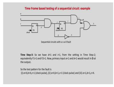
So, finally, a time step 1 you are going to get this one equal to 1, this one equal to 1. Now, basically this is equal to 1 so, this is equal to 0 and now I will just require a equal to 1. So, first stage basically you have to have a situation like this that is c equal to 1 will propagate the value second clock stage basically you have to apply it a equal to not require b equal to 1 and c equal to 1.
