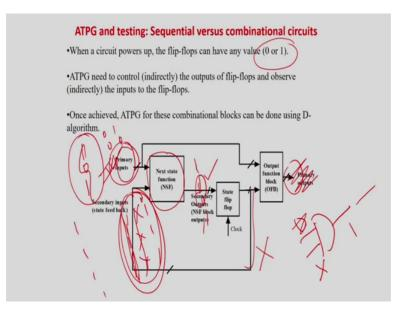
So, mainly concentrate on this part and other things can be easily extended to the output function block and very important these are the output of the flip flop. So, g are generally X, X means I do not know what are the values of 0 or 1, when a circuit powers up the flip flops have can have any values between 0 and 1, so, we make it X. So, all these inputs will be X and you can only control this and you can only observe this. In fact, these are non-directly observable lines.
