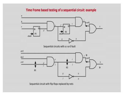
Now, we will take a more elaborate example to tell you what do you mean by testing of a circuit using time frame expansion method? So, assume that the let us take that this is the first the top figure solar circuit there are some flip flops and I have to test this circuit. So, basically we know that stuck at 0. So, what I initially do what is the algorithm for this also I tell you the algorithm to test it algorithm to generate the test patterns is very simple.
