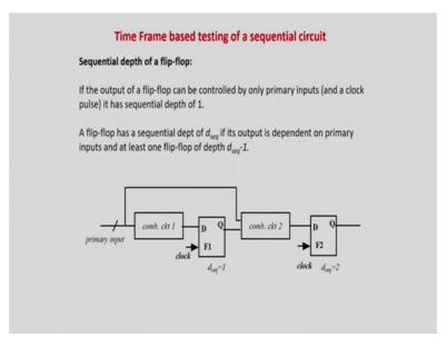
So, sequential circuit testing not only requires more time on the tester, but also the test pattern generation complexity is much higher. This philosophy you could have easily observed over here, because not only the sensitization of the fault propagation and justification requires to be done, but for that lot of secondary input lines has to be brought to them required values and for that again I have to do a lot of processing.
