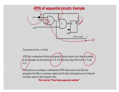
So, once you do automatically your e is going to become 0. So, this is what I was saying as an indirect control. So, if this would have been just assume if this would have been cut, so, what I could have done? I could have made a X equal to a equal to 1, b equal to 0 or in fact, I could have made b equal to X there is no problem and I could have made e or c directly equal to 0, sorry.
