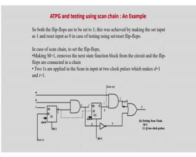
So, I have shown you in this figure so, I go to the test mode whenever you go to the test mode the primary inputs of this line and this line if you observe are cut. Primary input means the inputs from your or the main inputs which is the input for the next state function block or decoupled, but cut. So, this f 1 what I have shown is nothing, but your this one is actually f 1. So, what is this? This is the flip-flop with a multiplexer ahead.
