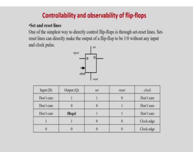
Now, we will come so, people started thinking about it they thought that this time frame based expansion method circuit testing will tell you anyway fail if the circles circuits are cycling. So, how they do? They started using the sorry the set and reset lines because, set and reset lines you can you can easily observe that if there was any kind of set and reset lines were there what I would have done it I would have made the reset line equal to 1, set line equal to 0.
