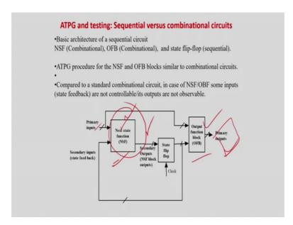
So, basically if you look at this diagram actually shows you the basic structure of a sequential circuit. So, you have the next state function block, you have the straight register you have the flip flops and is the output function block.
