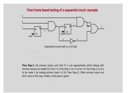
So, we require a 1 over here we require a 1 1 over here. So, what I require to do it over here first you have to make this line as a 1, I require a 1 over here so, two time steps ahead. So, I first require a 1 over here and I first require a 1 over here, I should get a clock pulse then the value will come over here. So, of course, to get a 1 over here I require a 1 over here. So, in the first time stage what I will do first time say I am targeting i equal to 1.
