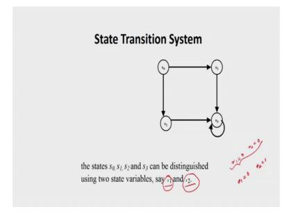
Now, to have this particular transition system and to represent the state, we need some encoding scheme and basically, we have going to use the state variables ok. So, since I am having four different states over here we need to state variable and we said these are  $x \ 1$  and  $x \ 2$ . And when we correlate this transition system with Kripke structure, which is used for your model checking then, this  $x \ 1$  and  $x \ 2$  may be considered as an atomic proposition of the system.
