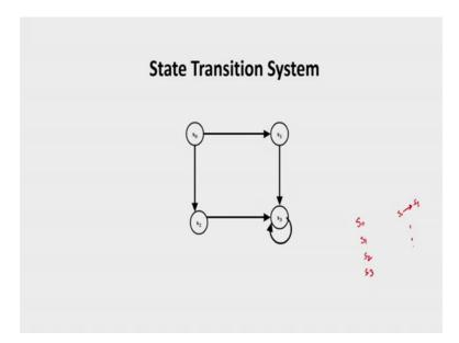
So, this is a state transition system so, we are having four states S0, S1, S2 and S3 and it is having some transition like say S 0 to S 1 like that, we having transition and this is a simple transition system that I am representing over here. And now, we are going to see how does information of the state transition system can be captured by BDD's or in particular OBDD's: Ordered Binary Decision Diagram.
