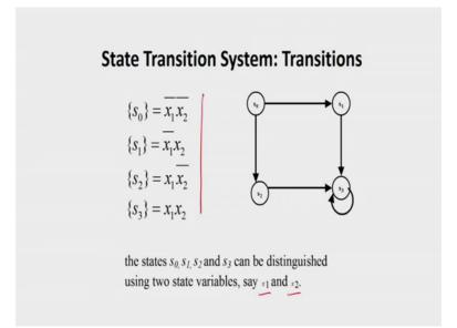
So, this is the state transition system we know this is the representation of 4 states and we are using these 2 state variable.
