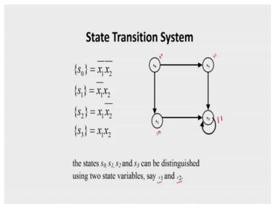
Now, for that we are using these 2 state variable x 1 and x 2. So, these 4 step can be represented like that S 0 the set S 0 is your x 1 bar x 2 bar; that means, the values of both the atomic proposition are the state variables are 0 0 over here; that means, we can say this is the state 0 0. S 1 is your x 1 bar x 2; that means, we can say S 1 is 0 1 S 2 is your x
