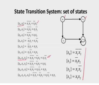
Now, for example, you just see that, we are having this particular same state transition system and a state encoding of these particular states are given is like that; S 0 is equal to x 1 bar x 2 bar, S 1 is equal to x 1 bar x 2, S 2 is equal to x 1 x 2 bar and S 3 is equal to x 1 x 2, you note these things.
