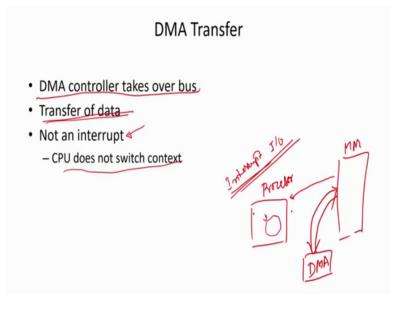
So, what basically, thus now basic info difference of what here is that DMA controller takes over a bus. So, now, system bus, basically data bus and address bus is used to connect the memory and along with that IO devices also. So, when we are using DMA controller then this control of this particular bus will be taken over by DMA controller; that means, processor is no longer going to use this particular bus, while DMA is transferring the information.
