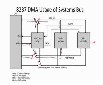
So, this is the scenario, you can see something like that; say this is the DMA controller, initially what will happen just you think that processor is directly connected to the main memory with this particular bus. This is the address bus, this is the, this is the data bus. So, processor is working with this particular memory.
