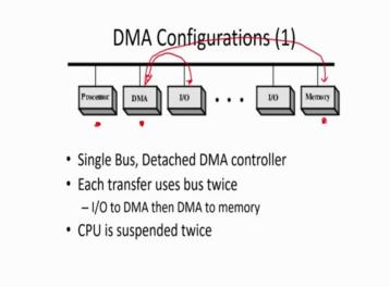
Now how you are going to connect those particular DMA controller. So, these are simple. So, this is a single bus, we detached DMA controller. So, in the particular user, see this is the processor. Processor is directly connected to the memory through this particular system bus. So, now processor can transfer information from memory.
