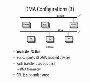
So, this is another configuration. So, again it is a two bus system; one is your IO bus and second one is system bus; that means, two system bus we are connecting to the memory to the processor, we are using a separate bus call IO bus and that IO bus that all the IO devices are connected to the IO bus and that IO bus is connected to the DMA controller. So, you will just see while again transfer of the information, the system bus will be used only once.
