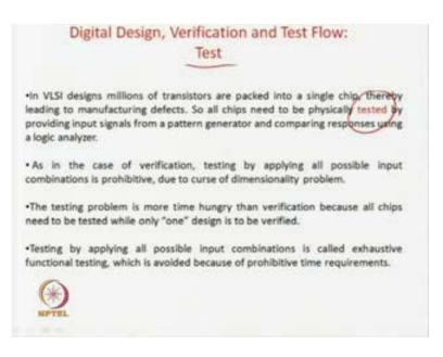
So, what we have to do? You have to test them by applying some test patterns. When the circuit it has been fabricated apply some test patterns. And you see they are proper or not. So, again if you have of dimensionally problem is there if you are to do for with 2 to the power of n p and where you have to apply for that for 2 to the power of n test factors. Now, we have to open for all the chips we have to do.
