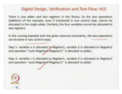
So, that is what I have told you? So, I mean in the running example there are 2 operations that is are doing in 2 control steps that is 2 control steps, because we have only 1 registers, 2 registers and 1 adder. So, first one you do this, second one you do this that is what has been told.
