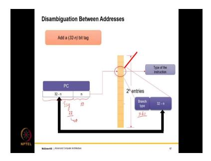
So, what we need to do is that the primary confusion that actually arises over here is because of the fact that we are using the lower n bits and the upper 32 - n bits they are not being used. So, it is possible that two addresses have the lower n bits in common, but the upper 32 - n bits are not common. So, we follow the same procedure which is that we use the lower n bits to actually address this table of  $2^n$  entries.
