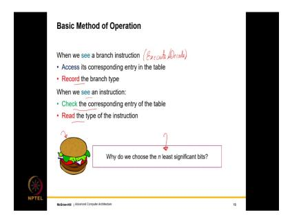
So, this is the basic method of operation where essentially we see a branch instruction, we see its PC, we access the entry in the table when we are seeing it, we record the branch type and when we see an instruction at fetch time.
