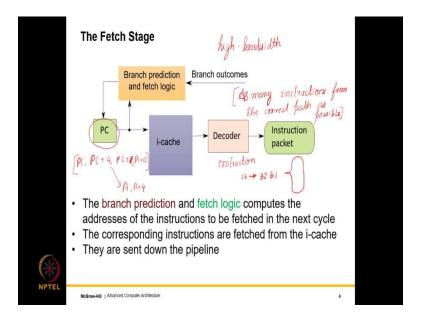
So, first a brief background. Let us look at the relevant part of the pipeline that discusses the fetch logic. So, the crux of the key state element that captures the fetch logic is the program counter, the PC, this points to the next instruction that needs to be fetched from the I-cache. So, in a RISC instruction set, the size of each instruction is fixed, it is typically either 4 bytes or 8 bytes. So, for the sake of simplicity, let us assume it is 4 bytes.
