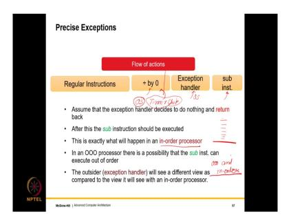
So, what we define is the notion of a precise exception? where the flow of action should be as follows we have a regular instruction before the div which means all of these. Then we see the divide by 0, then we load the exception handler and then we execute the subtract instruction. Alternatively, it is possible that maybe there was no divide by 0, but the operating
