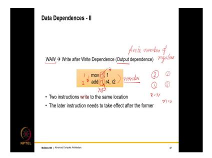
So now, let us move on to two other kinds of dependencies which were not causing an issue in order pipelines, but they will cause an issue in out of order pipelines. So, consider this piece of code whether write to the same register r 1. So, essentially the destination is the same, in this case, since they write to the same location and of course this is the program order it is not possible to reorder these two instructions, we cannot reorder them.
