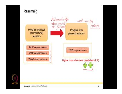
So, what does renaming actually do? Well, it takes a program with real registers, architectural registers that has 3 kinds of dependencies read after write dependencies, write after read dependencies and write after write dependencies. So, they have 3 kinds of dependency. And so then, the process of renaming which is automatically done inside the processor and nobody can see what is happening neither the programmer nor the compiler.
