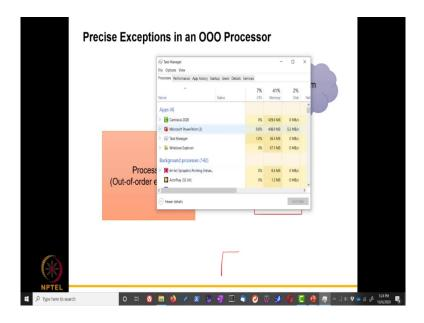
See if I have a single core what I am actually doing is that I am running multiple programs right program 1, program 2, program 3 etcetera on a single core. So, on a single core what will actually happen is that program 1 will execute till sometime. As we have said, we will have a timer chip it is very important to have the timer chip it is not a part of the operating system it is a separate piece of hardware.
