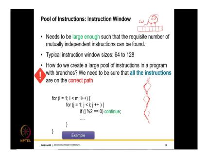
So, how large should the pool be? Well the pool is we will tell pool more as a kind of a conceptual entity and the hardware structure that stores this pool of instructions we will call it the instruction window which is nothing, but a simple queue of instructions.
