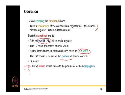
So, a few more details so, before entering the run ahead mode, we take a check point of the architectural register file, the branch history register, return address stack, such that the run ahead execution does not necessarily corrupt them. So, we do take a check point of these things, then we enter the run ahead mode. So, whenever we read a junk value, we add an invalid bit; all the instructions in the forward slices have an invalid bit, the inv value similar to the poison wit.
