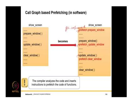
So, what we can do is that, there are two variants of call graph prefetching; one is in software and one is in hardware. So, we can do it in software first. So, this would require compiler intervention. So, what the compiler would basically do is that, it would add instructions to the code, where the instructions will go to the memory system and prefetch instructions and prefetch the data for instructions.
