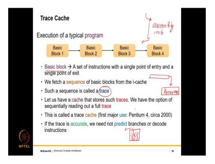
So, how does the execution of a typical program proceed? So, we typically execute programs a basic block after a basic block. What is a basic block? A basic block is a sequence of assembly instructions that has one entry point, in the sense you can only enter
