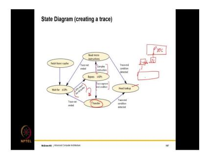
For creating a trace, so for creating a trace what we do is that, we along with a trace cache, we have a regular I cache as well. So, the processor diagram is that, we have a trace cache which we prefer; because it is faster, but we have a regular i cache as well, which is connected again to the memory system. So, we fetch instructions from the i cache, we wait for their micro ops to come and then the micro ops are temporarily buffered in the fill buffer.
