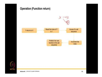
What is the operation of a function return? The operation of a function return is like this that, let us say that Y returns to X; at that point the present (Refer Time: 39:12), the present life of Y is over. So, we reset the index of Y to 1. So, the index of Y gets reset to 1; then we access X's call sequence.
