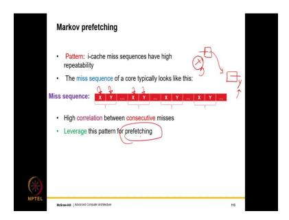
Next line prefetching is still only for the next line. So, the in a sense it is reach is limited. So, it is not really that smart a scheme, a slightly smarter scheme is Markov prefetching; in this case, we will have i cache miss sequences that are not necessarily to contiguous
