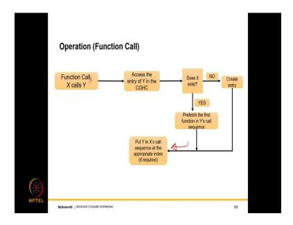
So, how does this scheme work? Well, the way that this works is a function call X calls Y; we access the entry of Y in the CGHC, which is the call graph history cache. So, does it exist or not? If it does not exist, we create an entry; if it exists what we do is, we prefetch the first function in Y's call sequence.
