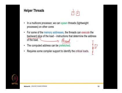
Something similar was proposed by another group called helper threads. So, here of course, we have multiple codes, not simple not a single one. So, in a multi core processor when you have multiple cores, we can spawn threads or lightweight processes and other cores. If you have one thread over here, we can spawn another spawn thread over there. So, let us assume in the program, there are some of these load instructions that are kind of prone to misses, they often miss.
