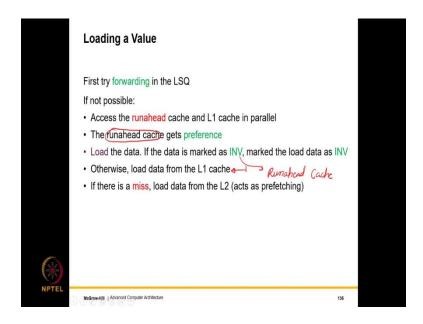
Loading a value, well loading a value will be the same first try forwarding in the LSQ; if it is not possible, we access the run ahead cache and I one cache in parallel, but of course the runahead cache gets preference. We load the data; if the data is invalid, we have marked the load data as invalid. So, otherwise we load data from the L I cache and if there is a miss.
