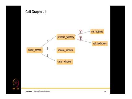
So, there is clearly a call graph, where each node is a function and each edge is an invocation of a child function. So, show screen first calls repair window, then update and then clear 1, 2 and 3 and prepare window call set buttons and calls set text boxes first 1 and then 2.
