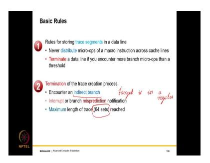
So, let us now look at the rules for storing trace segments in a data line. So, the first rule is that we never distribute micro ops of a micro instruction across cache lines. So, it is never the case that a single micro op is partitioned, a part of it is there in cache line one and a part of it is there in cache line two.
