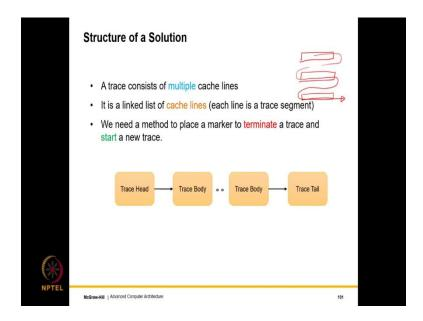
So, the structure of a solution is like this, let us consider a trace and let us assume that it consists of multiple cache lines. So, in this case, we are talking of a long trace that combines both the approaches. So, in this case, we can have multiple cache lines and we can say that a trace and was spans through all of this. So, this is like a linked list of cache lines, where each line is a trace segment, broadly speaking this is what we want to construct.
