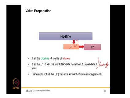
So, this is the typical architecture, where we have pipeline L 1 and L 2. So, if we restrict the changes to the pipeline; well then we nullify all the stores, we do not write anything to architectural state. If it is still the L 1, then that is ok; we can have invalid data in 1 and then it can be read back from here, but we do not allow any invalid data to go to L 2, because that would involve a massive amount of state management.
