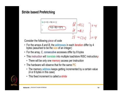
So, let us look at the simplest possible prefetching scheme, which is stride based prefetching; this is a typical example of a for loop and an array axis. So, if you consider arrays A and B; the addresses in each iteration differ by 4 bytes, where the assumption is that the size of an integer is 4 bytes.
