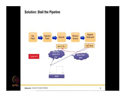
And in cycle N+2, this is the situation, and this is where a forwarding can be done where the r4 can be supplied and since we need the value of r4 now, well, the value of r4 can be happily supply to the EX stage. So, this is an example of a load use hazard as we just saw where a combination of interlocks and forwarding both actually solve the problem.
