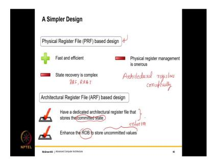
So, what we have seen up till now is the physical register file PRF based design, it is fast and efficient. However, there are problems, state recovery is complex, so, we need either a retirement register file or an RRA something of that type. Physical register management is hard, it is onerous, it is difficult. So, these are clearly some of the shortcomings of this scheme and these shortcomings broadly lie in the area of complexity.
