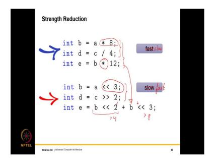
The next optimization is strength reduction. So, often we perform several arithmetic operations of this type. So, these arithmetic operations over here, they one is a\*8, / 4, \* 12. So, we very frequently also we compute the half of a value or the quarter of a value and because of this, we typically have multiply and divide operations of this type.
