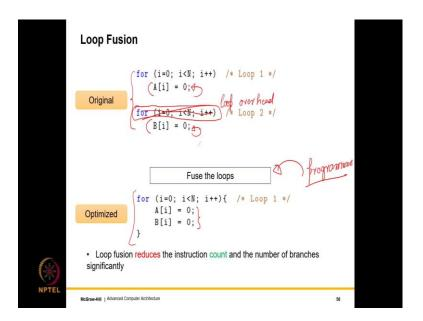
Another idea loop fusion well, let us take a look at these two loops. So, we have two loops, and we iterate from 0 to (N-1) and in the two loops all that we do is we set elements of one array to 0 and the elements of another array to 0 A i and B i. So, what
