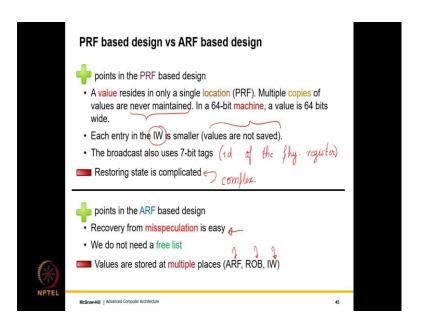
Let us compare the positive and negative points. Well, the positive points in the PRF based design which are plenty is that a value resides in only a single location. Multiple copies of values are never maintained.
