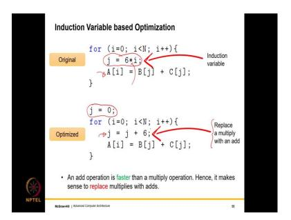
The other is induction variable-based optimization. So, in this case, the variable j which is derived from the loop variable i is known as an induction variable. So, as I mentioned the induction variable is derived from the loop variable. In this case, it is 6 \* i and then,
