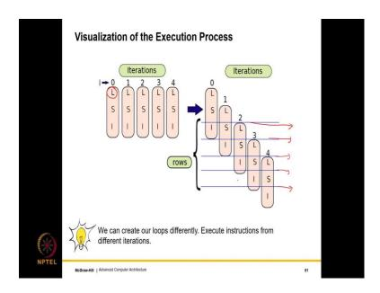
So, let us look at these three blocks across the space of iterations. So, we have a L block as you can see over here L, S and I. So, we have L, S and I for all the; for all 300 iterations, I am only showing for the first 5. So, I can write these in a different way, I can write L, S, I here, then I can write it the next iteration, I can just write it next, after that, then after that so, nothing stops me from writing it in this order, then I can create these rows as you can see.
