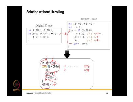
So, now, the we showed one way, one method of software pipelining, but the it turns out that there are other methods as well. So, the alternative solution that does not use renaming we will look something like this. So, let us first go from here to here. So, I have slightly expanded this C code such that one line roughly corresponds to one line of assembly or one or two lines, not more than that.
