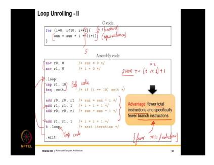
So, what we can do is that these 10 iterations can be fused into groups of two iterations. So, instead of incrementing i by 1, we can increment i by 2 and we can replace this sum operation with this which as you can see with the previous slide, this is equivalent. So, there is a degree of equivalence, it is the same basically what we are doing, it is just that we are doing more work within the loop and instead of 10 iterations, we have reduced the number of iterations to 5.
