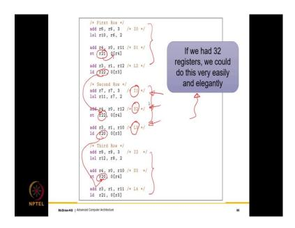
To do that, what we do is let us hypothetically assume that we have 32 registers, then we can do this very easily and very elegantly. So, what we can do is that we can in a sense create a new register r21 which stores output of S1. so, which S1 uses and then, r22 which is the load value of L2 and again, r 22 is used over here and again r20 is used by L3 which is again used by S3.
