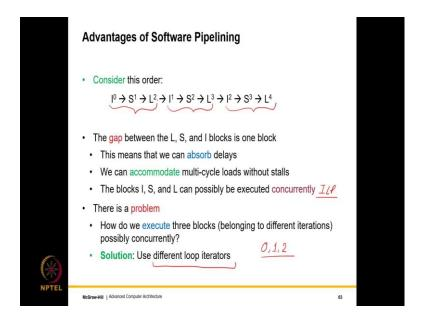
And these blocks so, if I were to just show this in a different way in a different manner what I can do is I can divide these into groups of three, if you would see that in each group we have blocks from different iterations and given that we have blocks from different iterations, what would essentially happen is that there is a possibility that we can execute them in parallel as long as there are no dependencies between them, this will further increase our ILP.
