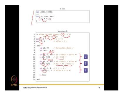
Let us now discuss software pipelining. So, we will use this piece of code as a running example throughout the lecture. So, in this piece of code, what we do is we consider two 300 element arrays A[i] and B[i] and we just copy the contents of array B into array A that is all that we do.
