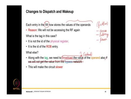
So, each entry in the instruction window gets modified. Previously, it was not storing the values of the operands. In this case, it is storing the values of the operands well, because there is no choice because that we have already accessed the register files, we are not going to access the register file. subsequently, hence each entry of the instruction window also needs to store the values.
