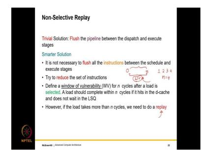
So, the trivial solution could be that we flush the entire pipeline or somehow we flush the pipeline between the dispatch and execute stages if it is doable, but this again is wrong and impractical and hard to implement. So, we should go for a smarter solution which is non selective replay. So, we will discuss three replay schemes non selective replay, a delayed replay and a token based replay.
