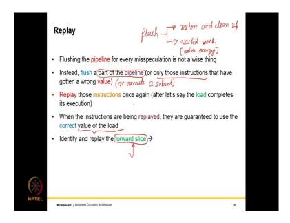
Well, one option we have for doing a replay which is to flush the entire pipeline. However, flushing the pipeline for every single miss speculation is not particularly a very wise idea; the reason being that it is flushing the pipeline is very expensive for two reasons.
