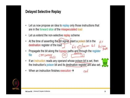
So, this method is known as delayed selective replay. So, here the idea is to replay only those instructions that are in the forward slice of the misspeculated load, they are the only ones that are executed once again and the rest are pretty much allowed to go through we will see how? So, here also orphan instructions are created, but we will have a new method a different method of actually dealing with them.
