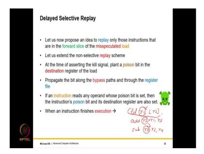
So, let me give an example let us say that we have a load instruction and this load has a miss speculation. So, we set the poison bit is this, then if we have an add instruction of this form, then we set the poison bit of r2 because it is reading r1. Then if you have a subtract instruction of this form, we set the poison bit of r3 because it is reading r2 so, on and so forth. So, pretty much along the forwards lies all the values get poisoned.
