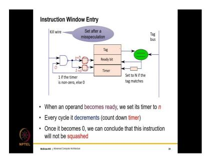
So, this is a special piece of logic where essentially what happens is for this piece of logic of the input is 1. We do not do anything in a sense we do not touch the timer we do not touch the ready bit. So, pretty much this circuit gets in activated if the input is 1.
