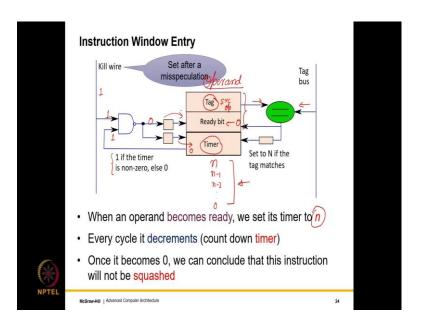
So, how exactly is this done? Well, the way that this is done is that the instruction window entry for every operand is augmented with some additional circuitry. What is that additional circuitry? Well the additional circuitry is that we store the tag over here.
