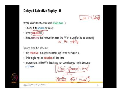
So, what do we need to do in terms of changes to the pipeline? So, when an instruction finishes execution, we check if its poison bit set which means after the E x stage. So, after the E x stage recall that we actually set a bit in the ROB indicating the fact that the instruction has completed its execution at this point we check if its poison bit is set if yes we squash it.
