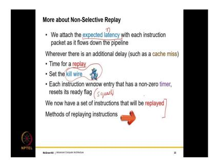
So, how do we do this? Well with each instruction if there is speculation we attach the expected latency which is essentially the value of n. Let us say there is an additional delay in sense this threshold of n gets breached maybe because we are doing latency speculation and we predict that it will hit in the d cache, but it actually misses in the data cache in that case it is a time for a replay.
