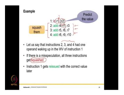
Let us consider the example of the speculation. So, let us assume that we have a load instruction. The load instruction loads from this address, the addresses stored in register r 2. Furthermore, assume that we predict the value the predicted value is stored in register r 1 which is the destination register of the load.
