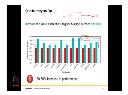
So, let us look at some of the basic results which sort of conclude a discussion on undergraduate computer architecture. The first is that if we take a regular 5 stage in order pipeline where basically if we look at the pipeline as a structure like this, instructions flow in, and they go through the 5 stages so, no instruction overtakes the other and then, they exit.
