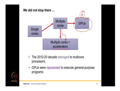
So, what people moved to was basically multicore processors. So, from single cores, they moved up, they moved up the hierarchy, up the chain and they went to multicore processors. So, instead of a single processor kind of on a chip, you have multiple small processors on a chip where each one of them can execute a program.
