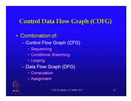
Let us just try to understand what that control data flow graph looks like because in various algorithms later on we may be using implicitly this c d f g that the what we have written in the HDL is captured in the form of a c d f g so that other algorithms operate on the c d f g. They do not operate on the file that you have written they operate on this intermediate representation.
