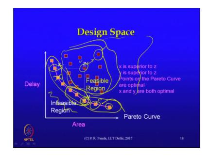
That is just to motivate the overall picture of a design space that exists for problems like this what we have indicated here is a two dimensional picture in which you have area on one axis and delay on the other axis considering that these are the parameters of importance when it comes to evaluating our design.
