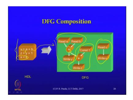
If I have a sequence of statements like this, this part of it is the first statement right. I have z equals y plus 1 that is the second statement, but there is an edge from the first output to the second input so that operators output is an input to the second operator that dependency is represented by introducing an edge between the two nodes.
