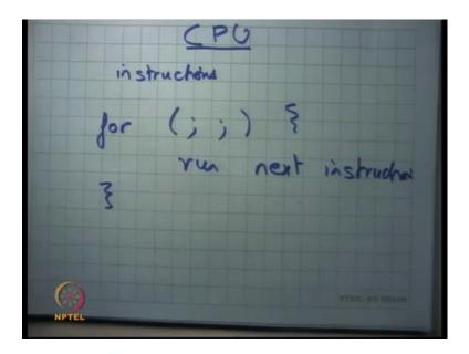
So, the hardware designers are basically implementing instructions and the software designers writing these instructions. And the logic of a CPU, is basically an infinite loop; if I were to write it and see let us say is just you know an infinite loop forever run the next instruction.
