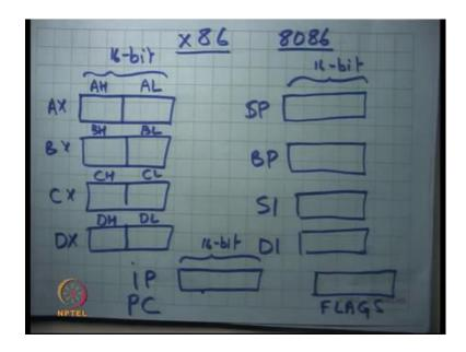
So, now let us concentrate on this on the x86 architecture. So, x86 architecture has a four data registers, they are called AX, BX, CX and DX; these are 16-bit in length in width, right. So, I am actually talking about the 8086 architecture, you know that was perhaps the first generation of these chips that we are using today, ok. So, you know let us say roughly in early 1980's or something.
