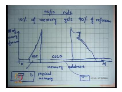
And, it is possible to do that because of this 90 10 rule I mean also call the 90 10 rule which basically says that this is a high amount of locality in accesses by a typical programs. So, programs typically 10 to access the same memory locations over and over
