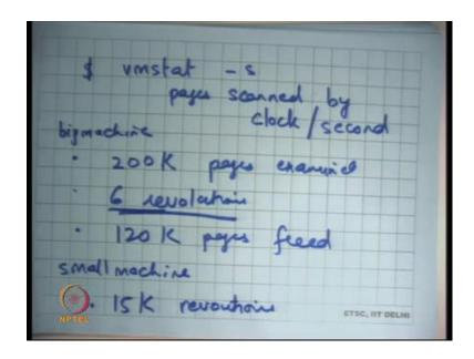
So, you know just as an example let say you know, I had a machine may find you know if you there is a command called vm stat on Sun OS. And, which allows you to check how many pages were scanned by the clock algorithm on operating system. So, clock algorithm is a commonly used algorithm in inside operating systems.
