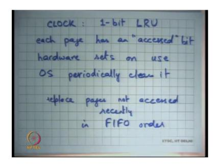
So, this algorithm is also called the clock algorithm, which is 1 bit, now can be thought of as a 1-bit LRU ok. Each page has an accessed bit or a reference bit right; hardware sets this one use and OS periodically clears it alright. So, the idea is that the operating
