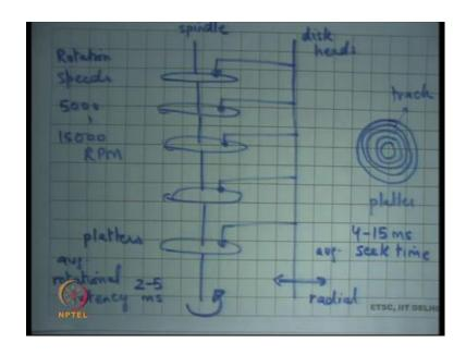
So, a magnetic disk is organized as a cylinder with such platters alright. So, these are this sort of these circular plates what is called platters all right, this axis is called the spindle. And the spindle is the axis of rotation right, so it just rotates right, and it rotates at a high speed.
