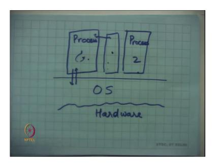
One of the system calls is the fork system call which actually creates another processes such that it is identical to the original process. These processes are more or less isolated from each other. So, if I am if I instantiate a variable in some process and I write something to it, it is completely in my private space as opposed to a variable that is instantiated in other process.
