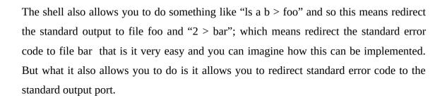
So, basically saying redirect the standard error; whatever is written to the standard error to the same resource that is being pointed to by standard output. So, that is the syntax for that one shell is 2 greater than and 1 depends on different shells, but let us say this is syntax for redirecting standard output standard error .
