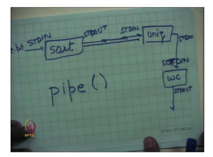
Ideally, what should have happened is that I should have had a way on my operating system to specify that here is a program sort, connect its standard input to file dot text and connect its standard output to the standard input of unique. And then connect the standard output of unique to the standard input of wc and connect the standard output of wc to whatever the standard output of the shell .
