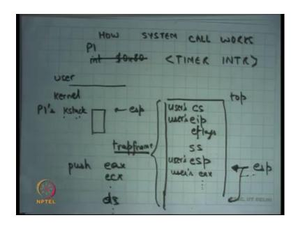
So, let us look at how a system call works alright. So, let us say this is user space and this is kernel space, and this is the process P 1 right and in the kernel space every process has a stack. Now let us assume xv6 is processes model so, every process has a separate stack kernel stack P 1's Kstack right.
