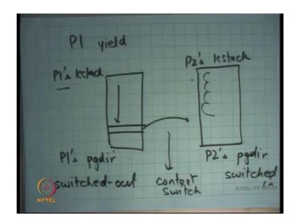
So, far we have seen a system call that that winds the kstack and then unwinds the kstack and then returns to the user mode, but yield system call which requires you to switch the process right, it is basically saying I do not want to run any more let somebody else run right. So, yield an example of a system call which will enter the kernel on P 1 kstack, but exit the kernel on P 2's kstack alright and in the middle this switching of stacks is what is
