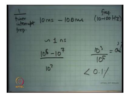
So, let me just first tell you know what kind of members are there, let us say 10 milliseconds to 100 milliseconds is the duration between 2 timer interrupts right. So, or 10 to 100 Hertz is basically the frequency typical frequency that you use for your timer interrupt right. On modern machines one instruction so, this is timer interrupt this is for one by timer interrupt frequency alright.
