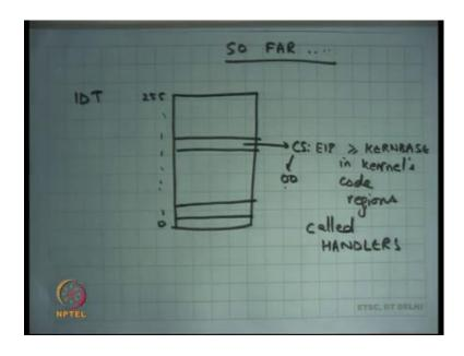
So, we have already seen this there is an interrupt descriptor table that has CS colony IB pointers CS has the last 2 bits as 0 0 which means it runs in privilege mode and EIP is somewhere in the kernels code regions so the handler gets called right. And, these pointers which are so initialized these are initialized by the operating system itself and we have already seen that the user is not allowed to overwrite either the IDTR which points to the IDT or the entries in the IDT itself.
