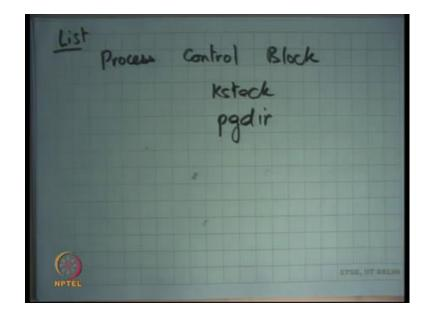
So, typically the process control block will have pointers to it is kstack and pointer to it is page directory and so there is a list of PCBs. So, this is a list of PCBs and the scheduler will pick one PCB and then switch to it is kstack and it is page directory and that is it, that is a context switch. So, all the information that was necessary to encapsulate the information exactly where that process got context switched out is available in the kstack.
