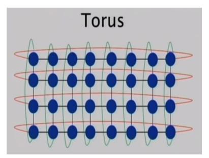
So it is not uncommon to have the torus connection where the last have a connection to the first torus so the last guy is right hand labor is the guy on that side okay. And similarly on this side the extension to this the notion of hyper cube connection.
