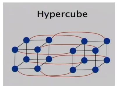
Which is again somewhere between taking is closer to full cross bar connection than bus but at the same time not incurring the entire cross and hypercube connection is also in some ways generalization of the mesh connection. So hyper cube for two nodes is simply a wire connecting right hypercube F4 nodes is wires connecting them in sub set of a grid a mesh.
