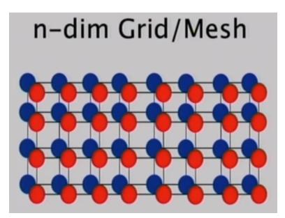
So this is 3D mesh in some implementation of mesh then you also have some additional wires so instead of just connecting it along the axis you also connecting to the diagonal there is another example of that where you connected diagonally. And so now and although there were other example likes CM which had a mesh connection mash power which is SIMD machine right.
