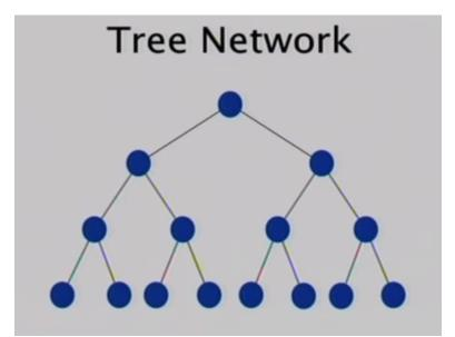
The next one would be the tree network by the way I was telling you about the parameters for interconnect one is of course the diameters what is the maximum time might take from node A communicating to node B. The other is the separation it is also called the bisection cost how many wires would you have to cut to separate it into two units meaning that now these set of processors have no power to that set of processors.
