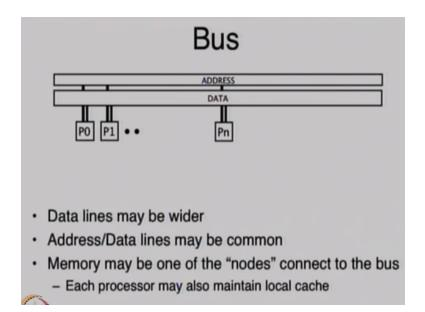
So that is a bus interconnect typically data lines would be much rider that than the address lines and the address and data lines can be common as we were just discussing for example in Ethernet and on the same bus may sit on memory loss. So you can send the address and the address may point in some memory and data will come out from that memory so some memory controller sitting on top of the memory deciding how to suck memory pins values and how to read values out of memory.
