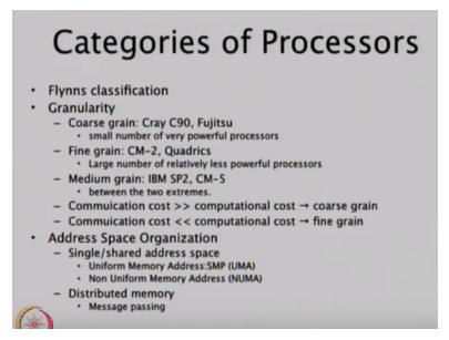
Let us move on to the history of parallel computers and will look at several of these axis Flynn's classification SIMD or MIMD or a combinations what is the size of the processor what is the granularity of the processing elements there may be lots of weak processors or a very few strong processors very powerful processors their address space organization and whether there are shared memory and receive it.
