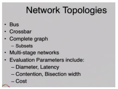
So typology is in general will be bus which is for example Ethernet was lots of notes have bus is going to have lots of notes and different notes will look in that bus okay normally in the parallel computer context there will be address bus as well as the data bus put address on to the address bus and the data consult from the data bus or you put the data to the data bus and addressing to the data address bus.
