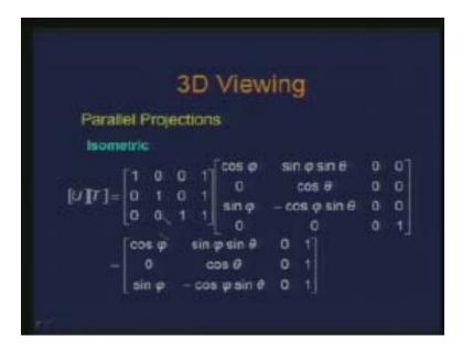
Similarly I have the foreshortening in Y the square of it given here and foreshortening in Z. Now I impose the constraint of the transformation to be isometric which in turn means
