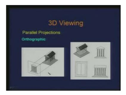
Here we notice that these are the projectors, this is the projection plane and these projectors are parallel to each other and they are also perpendicular to the projection plane and these are the various views we can get of this object such as the front view, the top view and the side view.
