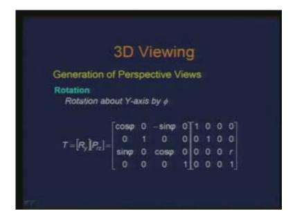
I do a rotation before I take the perspective transformation and now I am always doing perspective transformation which is a single point that is one point. Now I do a rotation about y axis by an angle phi. So the total transformation is basically the rotational transformation and the projection transformation which is this multiplied by this.
