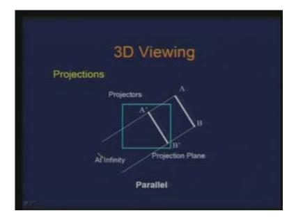
Now the other type of viewing projection is the parallel projection where we have this projectors coming out the object AB parallel to each other and this is again the projection plane. So, in effect what we get is the center of projection now moves to infinity. It does not meet at the point which we will call it as the center of projection. So this is parallel projection and we basically looked at the various types of parallel projections.
