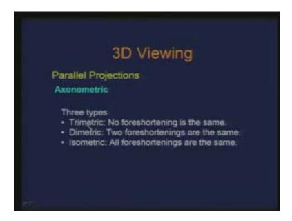
Therefore for instance I can basically define three types of axonometric projection; trimetric where no foreshortening is the same. So  $f_x$  is not equal to  $f_y$  is not equal to  $f_z$ . In diametric two foreshortenings are the same out of these three and in isometric all the foreshortening are the same.
