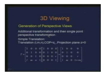
Hence let us consider a simple transformation like translation. If I apply a translation by the offset I m n to the object and again I consider the center of projection located at Z is equal to c and the projection plane Z is equal to 0 then I just concatenate these two matrices the translation matrix and the projection matrix and this is what I get.
