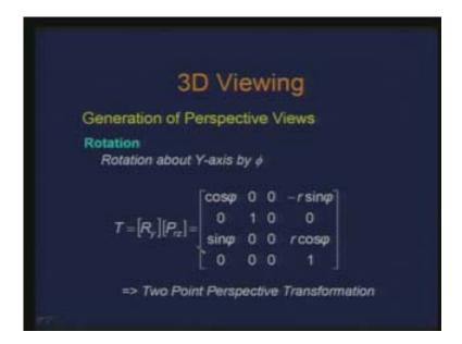
And if I see the resulting matrix this is what I get. In the last column we considered single point perspective. The only thing is I applied a transformation of rotation before I gave the perspective transformation. So now this gives me a two point perspective transformation. Therefore in this way I can have a two point perspective transformation using single camera.
