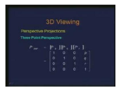
Now I can further extend this idea where all the three entries here are non zero p q r. And once again this can be obtained as concatenation of the three one point perspective
