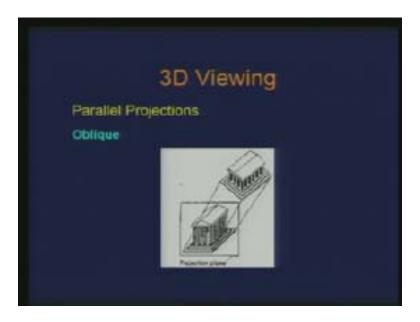
This is again an example here, here these projectors are not perpendicular to the projection plane. And again the motivation of having oblique projection is to add the element of 3D viewing, to make it look like a 3 dimensional object. So this is the example of oblique projection.
