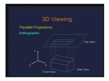
For instance, we looked at the orthographic projection where we basically have an object and the projectors are parallel to each other and they are perpendicular to the principle planes which are actually planes perpendicular to the principle or the coordinate axis. So this is for instance gives us the top view the plane which is perpendicular to the y axis and similarly the front view and the side view we get.
