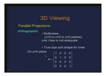
Mathematically we can get this projection again using as a matrix transformation. Therefore this matrix P basically gives as an orthographic projection on Z is equal to 0 plane. What we get basically is this third column and all the values are 0. So we can represent this orthographic projection again as a matrix transformation. So the property here we have basically preserves the true silent shape for the object. So these are the examples.
