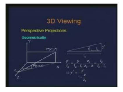
Using a matrix form of transformation we know what we got. Now let us try to see geometrically. So here is your center of projection along the Z direction Z axis located at  $Z_c$  and this is your point P(x, y, z) and we are looking at projection on Z is equal to 0 plane meaning (x, y) plane. So I basically project this point through the center of
