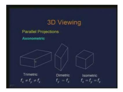
As an example here we have the trimetric projection where  $f_x$  is not equal  $f_y$  is not equal to  $f_z$ . This is diametric so you that this basically equals to this if I had taken the object to start with as a queue. So when we observe the foreshortening these two directions are the same. And in isometric I have all the foreshortening. What basically happens here is that
