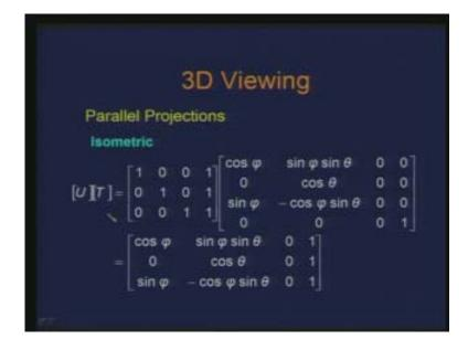
Again I have the three unit vectors and this is the transformation. Once I apply the transformation on to these three unit vectors the modified or the transformed unit vectors are dmos. So the first row gives me the transform unit vector in X, the second row gives
