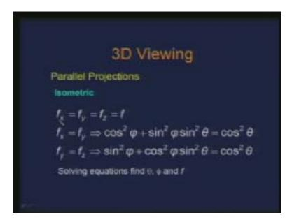
Now I have these three equations where I can solve it for pi, theta and f. So basically it can give me the amount of rotations I should be performing in order to get isometric projection for a given value of foreshortening. Now we move on to the other type of parallel projections. So what were the observations we had in the axonometric projection? It was that the projectors were parallel and they were perpendicular to the projection plane. Now we relax one of the restrictions.
