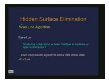
Here is another method of hidden surface elimination which is actually a combination of z buffer and scan line conversion of polygons. It is a scan line algorithm basically and it is based on scan line coherence across multiple scan lines or span coherence. When you scan convert a polygon then you get span or portion of the scan line within different polygons. For a given scan line you will have a span of this scan line contained in different polygons.
