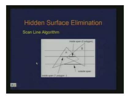
So in some sense we are exploiting the span coherence and for each span as we observed a visibility test may be required as we observed particularly when there are more than one polygon which are intercepted the span. You may have different kinds of spans. There is a span which is inside only one polygon. This is the polygon A and this is the polygon B and this is the span. For this particular scan line this span is contained in one polygon.
