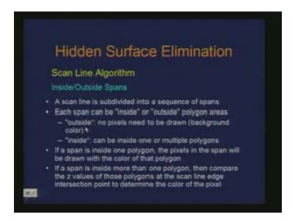
So the outside span is that no pixel needs to be drawn or you draw the background color because it is not contained in any of the polygons. The inside span can be either inside one polygon or more than one polygon.
