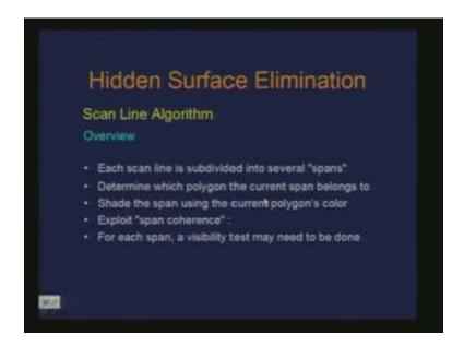
Determine which polygon the current span belongs to, shade or color the span using the current polygons color or shade. So, in a sense we are actually exploiting the coherence within this span. Once we establish that this span is contained in a particular polygon and this is the polygon which is to be displayed then all the pixels or all the points along that span could directly be rendered.
