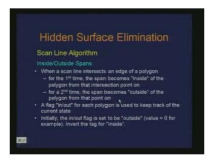
So if a span is inside one polygon the pixels in the span will be drawn with the color of that polygon and if a span is inside more than one polygon then you need to resolve for the visibility which may be through the z value of the polygons. So the question is if you are talking about this labeling of inside outside spans or inside one polygon inside multiple polygons how do we do that?
