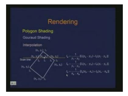
So here if I have the horizontal axes as X and the vertical axes as Y then my interpolation parameter T kind can be just Y.
