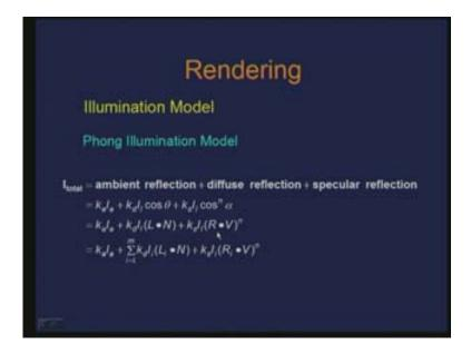
So using these two vectors we can compute the specular component of the illumination. And in fact we also looked at how we compute reflected vector in terms of L and N. and there is also this specular coefficient which again captures in some sense the material property on which this specular component is computed.
