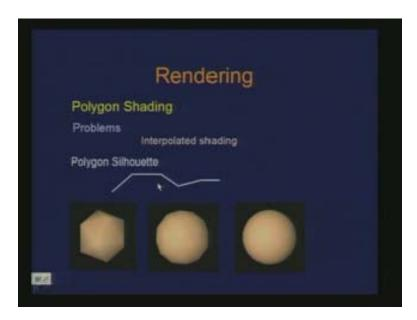
No matter what kind of shading you do for the interior part of the object this boundary is visible. Therefore it does indicate that the object is polygonal. For instance, if I have a very coarse polygonal representation of the spherical of object this is what I would see and this is shows that it is a polygonal representation where there are sharp changes. And in fact if you see here carefully these are the boundaries and that is where you still see the Mack band effect.
