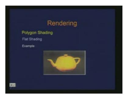
So as a rendering or the display of the object in terms of its realism is not as realistic as we would like to have it particularly when we know that this was derived from the continuous surface representation, parametric representation. One option could be to have very small polygons then try to use flat shading for each of those small polygons. Clearly there is an overhead but then you have to treat so many polygons.
