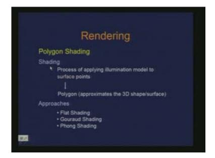
There are basically three approaches which are used for shading polygons. One is flat shading, then gouraud shading and phong shading. For flat shading we actually have one illumination or intensity computation for the entire polygon. The polygon is assigned one intensity. That is where we have constant shading for the polygon. That is why sometimes flat shading is also called as constant shading.
