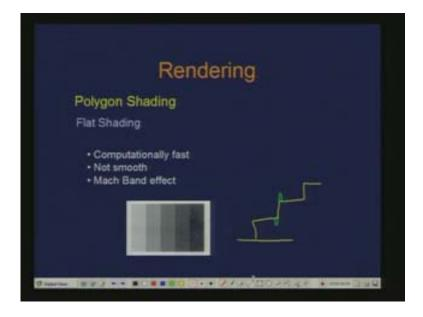
What you see here looks like this particular point had lower intensity than this band and this point of point in the vicinity this border has higher intensity. Therefore these boundaries are perceived to have this artificial brighter spots and darker spots. This is due to the perceived intensity from our visual system. When we are talking about the flat shading flat shading is shading where we have discontinuity at the boundaries. Therefore
