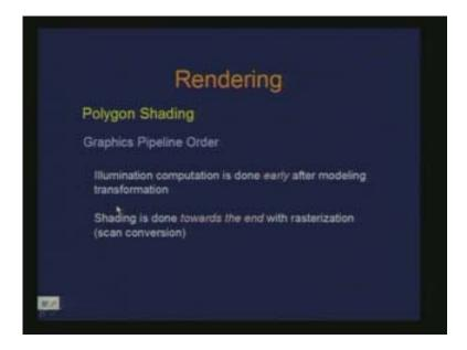
This is how these computations are located with respect to the rendering pipeline.
