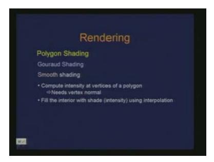
Now instead of having face normal I need a vertex because I am going to compute the intensity at the vertices of the polygon. And once I have done this, that means I have computed the intensity at the vertices of the polygon I can then fill the interior with the shade of the intensity using some interpolation.
