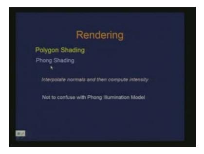
Phong shading is basically a polygon shading model which is different form phong illumination model. As in the case of gourand shading here you have normals at each of these points.
