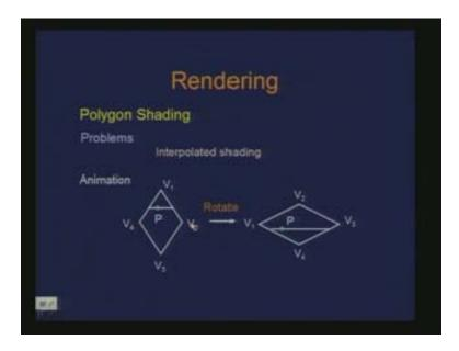
Here we are saying that for this computed intensity if I am not changing anything for the light source, you are rotating the object. If I am just rotating the object orthogonal to the light source why would there be a change. So unless I am changing with respect to the light source if I am moving away from the light source then I may want the intensity which is computed for the point to be different.
