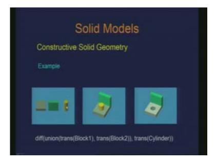
Now, is it unique? This CSG representation is not unique. You can construct this in different ways. Now looking at this as a chain of transformation accompanied with the Boolean operations I can actually represent this as some sort of a tree.
