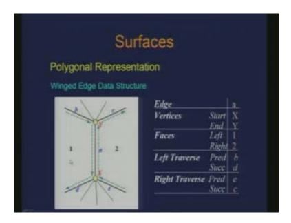
This is the connectivity link between points. That is what establishes the connectivity of a mesh. So I just traverse through that and I can derive information about the polygons which would be adjacent to an edge or sheared by that edge. And I also have the explicit information about what vertices the edge constitutes so X to Y I know that.
