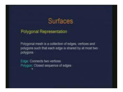
So the explicit representation we looked at is basically a way of representing a polygon as a collection of individual vertices to form that polygon. And you write it in a sequence so that the last edge which will be formed is between the last point and the first point. Therefore the coordinates of each of these vertices is given explicitly.
