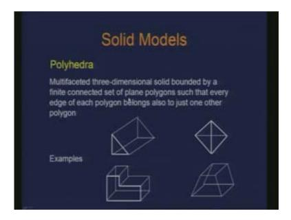
But if you look at each of these edges these are exactly sheared by the polygons. What are the elements which we use for defining polyhedra? We have a vertex, we have the edge and we have the face. This is what we need for boundary representation of a solid. And we also have the angle which is formed at the edge between the two faces of the polygons which we call it as Dihedral angle.
