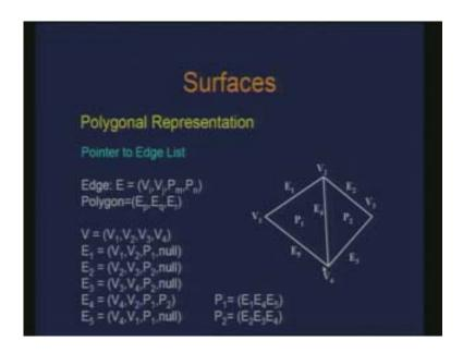
A slight variation could also be done if I am also interested in finding out holes. Hole is also some sort of a boundary. May be you need to have an orientation in which you traverse the list. So, this is in order to distinguish between hole and a boundary. You can always get hole and boundary using this data structure.
