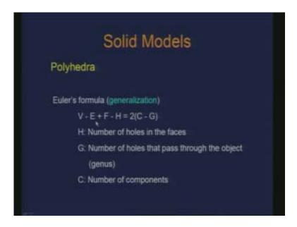
For instance, sphere has a genus 0, torus has a genus 1 and that is what we mean here and C is the number of connected components. So, if you want to incorporate this information then the Euler number is modified like this. Here is another example, I have a solid like this so this is a through and through hole and this is just a hole at the top and it is not a through and through hole.
