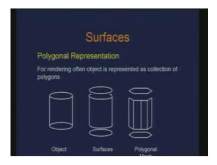
Therefore you primarily get the point clouds for which you establish the connectivity and form triangles or any polygons. That is the kind of data for which you would like to again use a polygonal representation. So what we basically looked at is that if there is an object of this kind it could actually be made of several surfaces. So in this case there is a surface which is the sides of the object and then there are caps of the cylinders.
