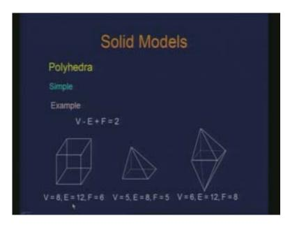
Similarly, you have for tetrahedron which is also simple polyhedra where the condition of Euler number getting satisfied. The polyhedra which we are considering do not have holes on its faces and there is not a hole through and through in the object, it is a closed surface solid.
