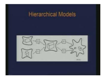
This shows some sort of a hierarchy in the modeling process. So what we are looking at is some sort of a graph a directed acyclic graph bag which will have the leaves as simple primitive objects for the model, these edges are the transformations, again we get some aggregated model and again using some transformations we build our world or scene.
