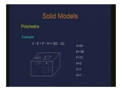
Now if I count the total number of vertices it comes out as 24 and number of edges as 36 and number of faces as 15. Now the number of holes on the faces is 1 2 3. The connected component is 1 where the whole thing is connected and genus is 1. There is one hole
