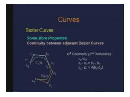
Now if you look at the relationship of the control points in the two curves  $c_0$  is the same as  $b_3$  satisfying  $c_0$  continuity and  $c_1$  minus  $c_0$  is equal to  $b_3$  minus  $b_2$ . Basically all it says is, symmetrically if you want to see that this leg of the polygon in the first case is the same as this leg of the polygon and they are collinear. Whereas if you see here the
