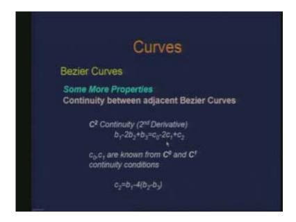
Now you see that  $c_2$  is given as  $b_1$  minus  $4(b_2$  minus  $b_3)$  because  $c_0$  is  $b_3$  and again  $c_1$  minus  $c_0$  is the same as  $b_3$  minus  $b_2$  so that gives you  $c_1$ . Hence you just use that information to get  $c_2$ . So how does it look visually? Now I have the first curve  $P_1(t)$  given as this through  $b_0$   $b_1$   $b_2$   $b_3$  and the second curve given as  $P_2$  through  $c_0$   $c_1$   $c_2$   $c_3$ .
