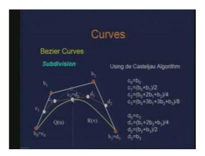
And further application gives me the point here the point here. One more application gives me the point on the curve. And this is the point where this subdivision is taking place and that is where I am subdividing the curve.
