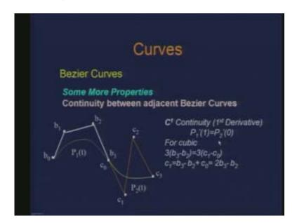
Here, again if I have the first curve defined through the Bezier polygon  $b_0$   $b_1$   $b_2$   $b_3$  and the second curve  $c_0$   $c_1$   $c_2$   $c_3$  then here if you look it looks smoother. The transition from one curve to the other curve is smoother. And in order to establish this I would require
