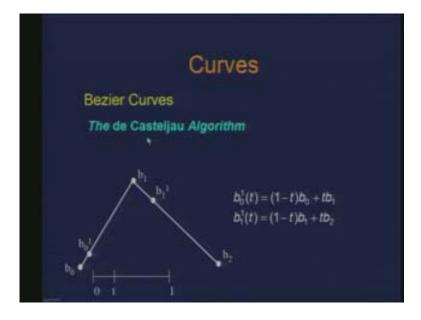
This de Casteljau algorithm basically works using linear interpolation. So the idea there is that if I have the parameter t is defined between 0 and 1 so for any value of t I can locate a point on the curve by successive application of linear interpolations. That is the underlying idea about this algorithm which basically means that if I apply a linear
