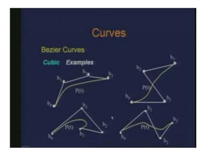
Then we actually started looking at a different way of constructing these Bezier curves. One was using Bernstein polynomials just as a basis or blending function and there is another way of constructing these Bezier polygons and that is due to this de Casteljau algorithm.
