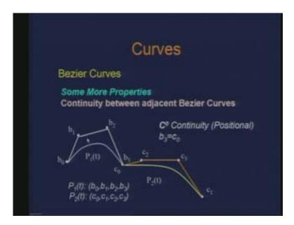
Now if I am talking about the continuity at the junction point of these two curves the first thing I can look at is the positional continuity where the first point of the second curve should match with the last point of the first curve because that is the minimum requirement of the two curves to be joined. So we are talking about positional continuity which we call as  $c_0$  continuity. This is the first curve.
