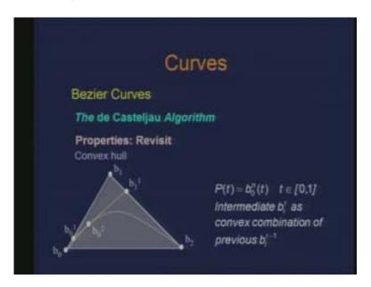
Now let us try to see the same thing in de Cateljau algorithm formulation. So once again if we just look at the construction mechanism which is to use successive application of linear interpolation, so what do I have is, this is the definition of the curve, this bn0t finally gives me the curve P(t).
