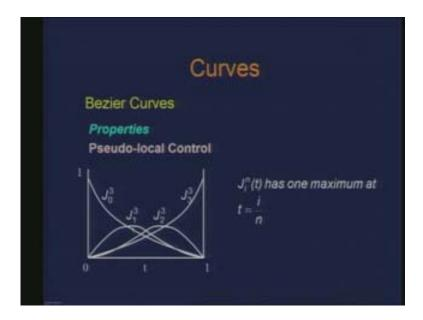
Basically it means that if I move a particular control point of the Bezier polygon then what is the kind of influence I have to the curve?
