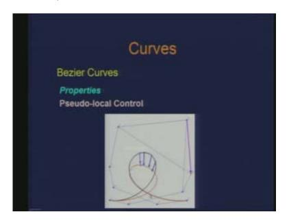
So this is important to know from the point of view of designing curve. So as a user you should know the range of influence to the curve when I am going to change a particular point, this is useful from the interface. Another property is variation diminishing. This is for the case of planner curves. When I talk about space curve they become plain. So here it says, for planner curve no straight line intersects a Bezier curve more number of times than it intersects the curves control polyline.
