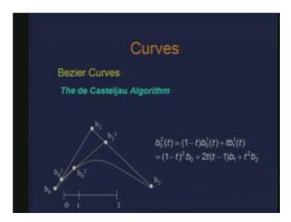
So this construction is due to the person called de Casteljau who gave this algorithm of constructing parametric curves which were later on called as Bezier curves because Bezier came only in 1970s whereas de Cateljau came in early 1900s. So he had already done this. So the same construction using Bernstein polynomial actually can be obtained by a repetitive linear interpolation.
