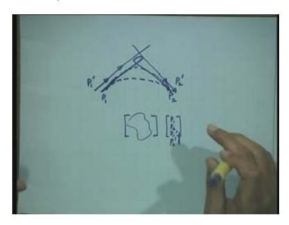
We also observe that the end conditions which are specified also affect the shape of the curve. It is also a control in terms of the kind of spline you would like to obtain. For instance, we observed that these are the four commonly used end conditions. So, if the two end tangent vectors are specified we say that these are clamped end conditions and that is what we have basically studied so far.
