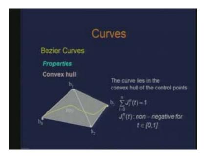
Now we will use the properties of our Bernstein polynomials. If I have to have a point or a curve within the convex hull of these control points would actually mean that the point which is computed using the convex combination of those set of points or the control points. And how do I get these convex combinations? It is by these two properties.
