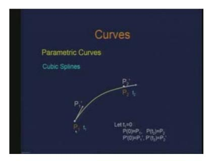
So given these conditions as input also the running parameter  $t_1$  and  $t_2$  we construct a spline which passes through these points and satisfy the tangent vector conditions at the two end points and that is what we obtain cubic splines for. Now, if we extend the idea between the two points to any n number of points so there we are concerned of having these tangent vectors determined by certain constraint which is imposed on the curve rather than this being specified by the user.
