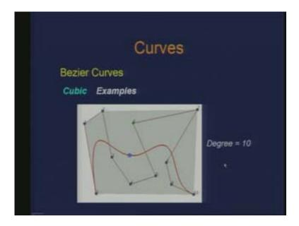
Therefore, degree and the number of control points are directly related. Now let us try to see certain properties of these Bezier curves. The first thing we observe just by the plots of various curves we have seen is that the Bezier curve interpolates to the end points. The first control point and the last control point it passes through.
