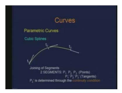
Therefore again only the two end tangent vectors are specified if desired and the intermediate tangent vectors are determined or computed using some continuity condition. And what we used was that the c2 continuity condition in the case of a cubic spline where we say that the second derivative is the same at the joining point.
