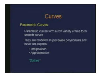
By free form we basically mean, a form which is not constrained by its representation. And these parametric curves basically offer the flexibility where we can freely change the form when we draw a curve. They are actually modeled as piecewise polynomials and we have two aspects; one is that they could be interpolating curves as we observed in the case of cubic splines the interpolating cubic splines or they could be approximation to a certain shape which is defined by certain input.
