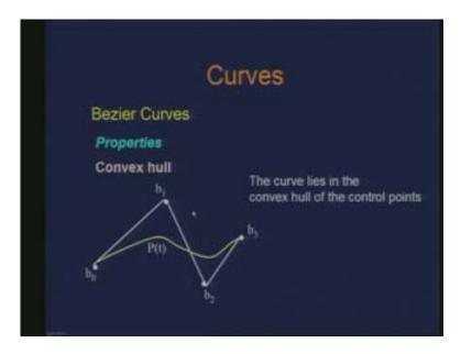
If I have this basic curve here defined as P(t) coming from the control points  $b_0$   $b_1$   $b_2$   $b_3$  then this curve is going to reside inside the convex hull made by these points  $b_0$   $b_1$   $b_2$   $b_3$ . This means first of all let us try to construct the convex hull of the control points which looks like this, this is the convex hull, all it says that the curve is going to lie within this.
