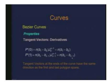
Now again let us say I take the case of a cubic Bezier curve where this is my Bezier polygon and I just basically write the first differences as these legs of the polygon. This is delta  $b_0$ , this is delta  $b_1$  and this is delta  $b_2$ .
