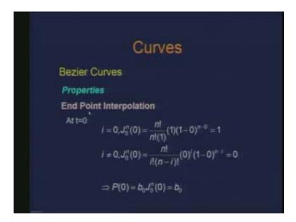
That can easily be seen here. If I just substitute for t equal to 0 what happens to the j and i? Here I see that it becomes 1 and the rest becomes 0. So it immediately gives us P at 0 as this and all the other terms are cancelled and I get this as  $b_0$ . It is just a simple substitution.
