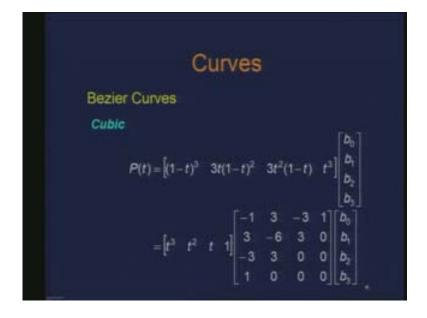
This is the monomial form of the coefficients 1t t power 2 and t power 3 so I get a matrix representation for cubic Bezier curve. Now these are the examples. So you have  $b_0$   $b_1$   $b_2$   $b_3$  and this is the corresponding Bezier curve.
